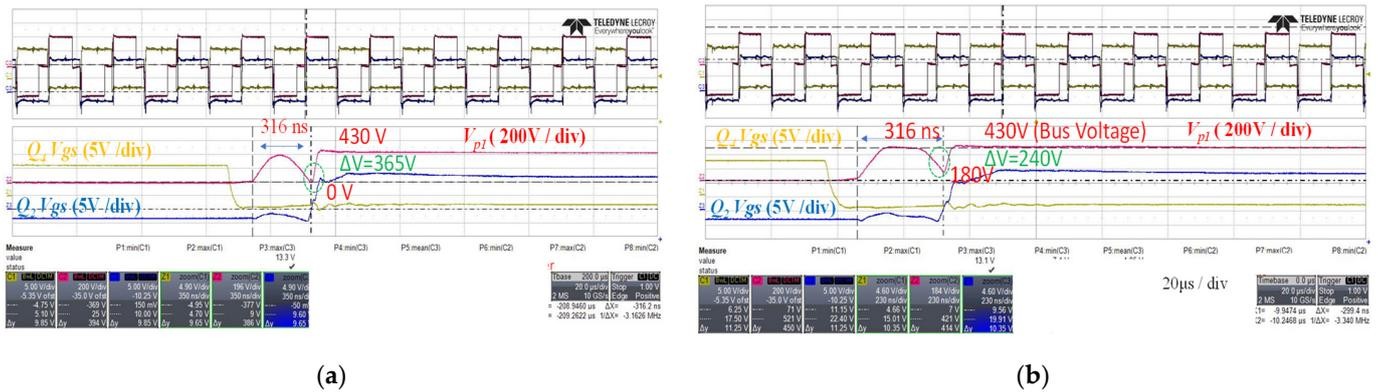
Figure 17. Experimental transformer waveform with a fixed dead time. (a) At half-rated load. (b) At full load.
