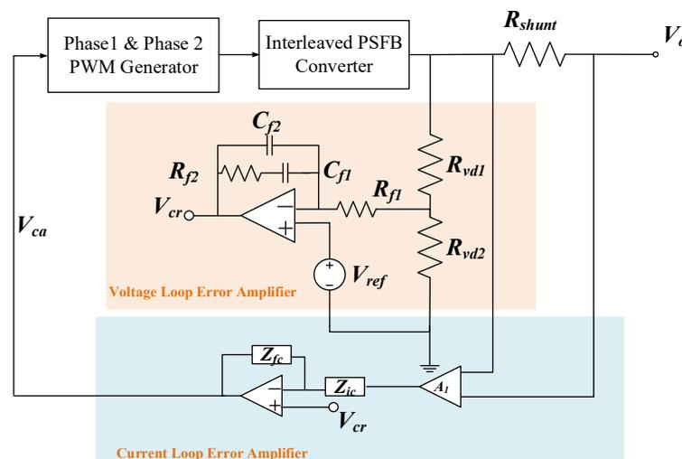
Figure 5. Dual-loop controller of the proposed PSFB.
