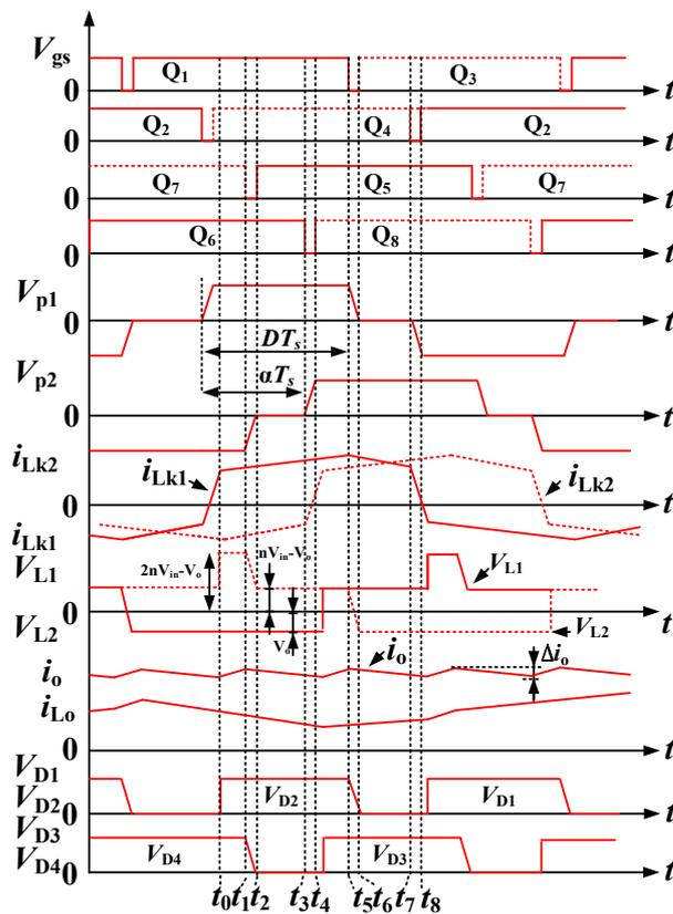
Figure 3. Key waveforms of the proposed PSFB converter.
