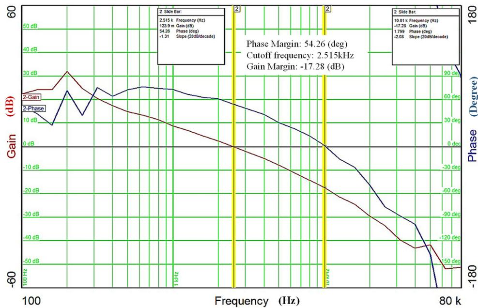
Figure 20. Frequency response of the PSFB converter.
