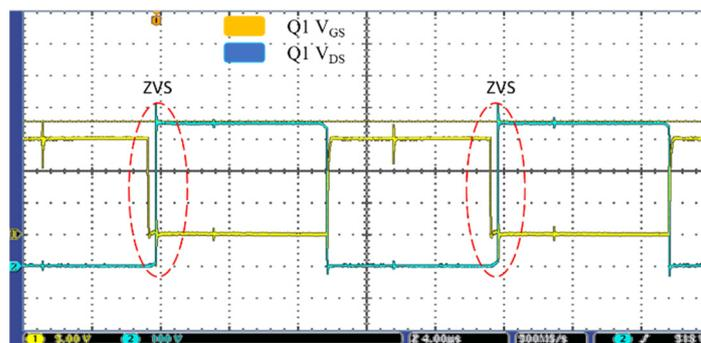
Figure 19. Zero-voltage switching (ZVS) waveforms of  $Q_1$  at a 12.5A load.
