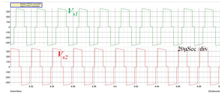
Figure 12. Simulated waveform of the secondary voltage across the transformers.
