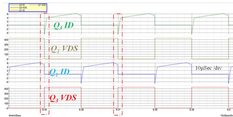
Figure 13. Simulated waveforms of the drain current and drain-to-source voltage across the MOSFETs in the same bridge leg.
