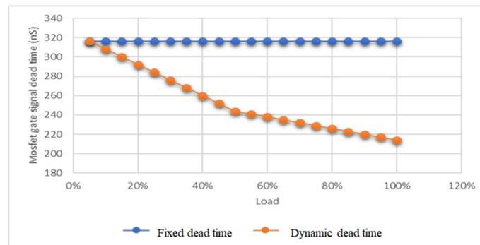
Figure 9. Fixed dead time and dynamic dead time as functions of load.
