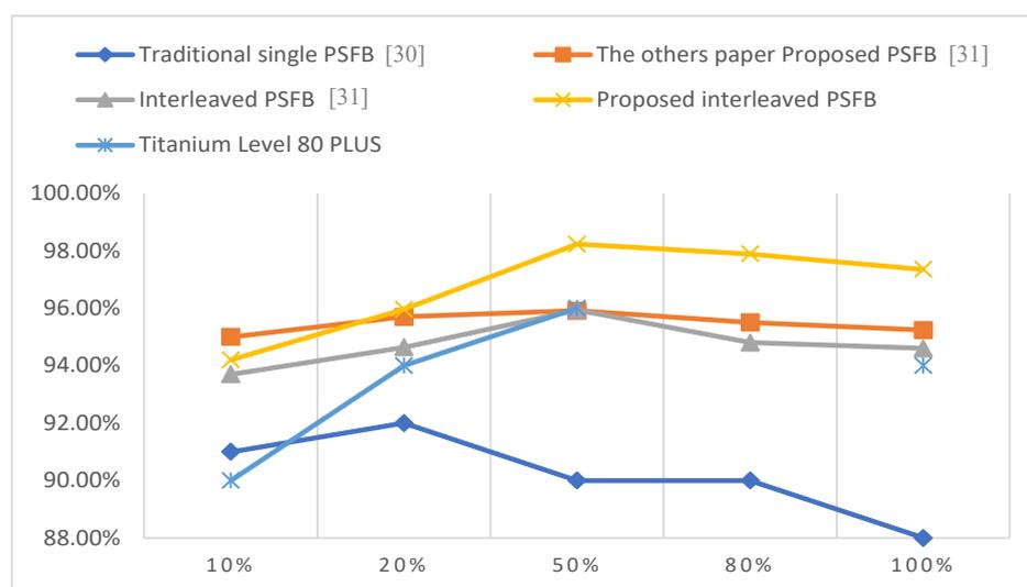
Figure 22. Measured conversion efficiency curves.
