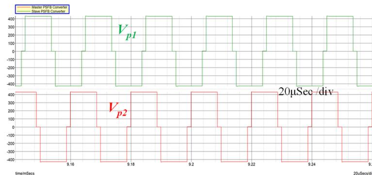
Figure 11. Simulated waveforms of the primary voltage across the transformers.
