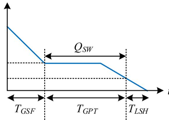
**Figure 8.** Gate turn-off voltage and time intervals.
