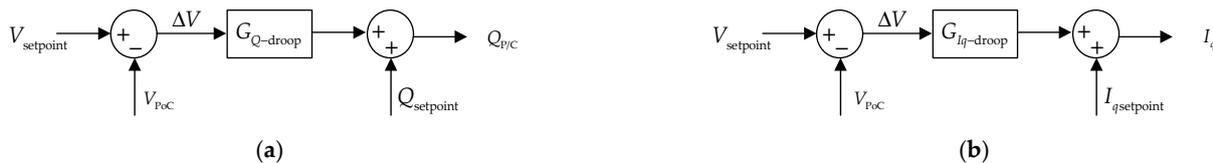
**Figure 4.** Proportional control based reactive power control strategy at smart converter: (a) Voltage Q-droop control; (b) Voltage  $I_q$ -droop control.
