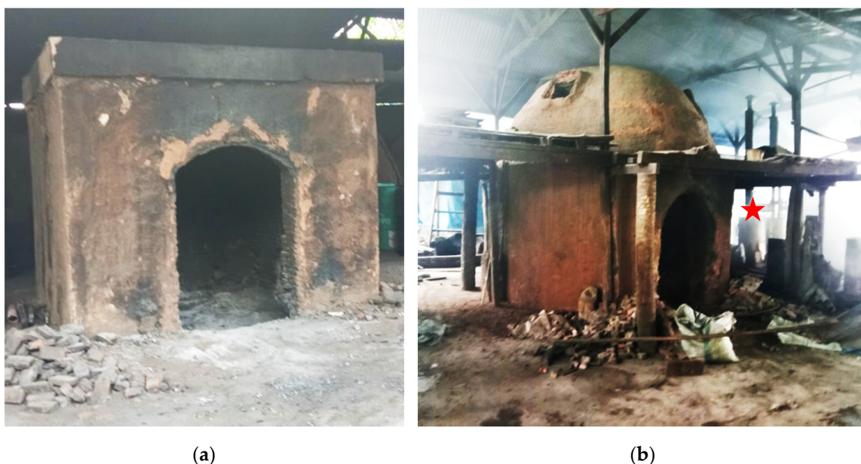
Figure 1. (a) Box furnace and (b) dome furnace. The red star symbol at (b) is the condenser system.
