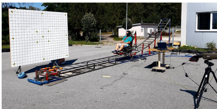
Figure 6. Test stand for crash tests at low speed.
