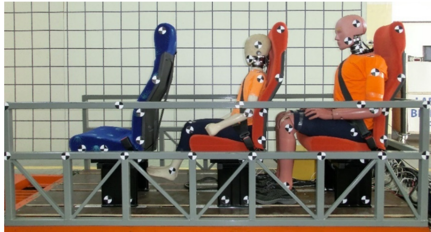
Figure 4. Test stand located at the Automotive Industry Institute in Warsaw.
