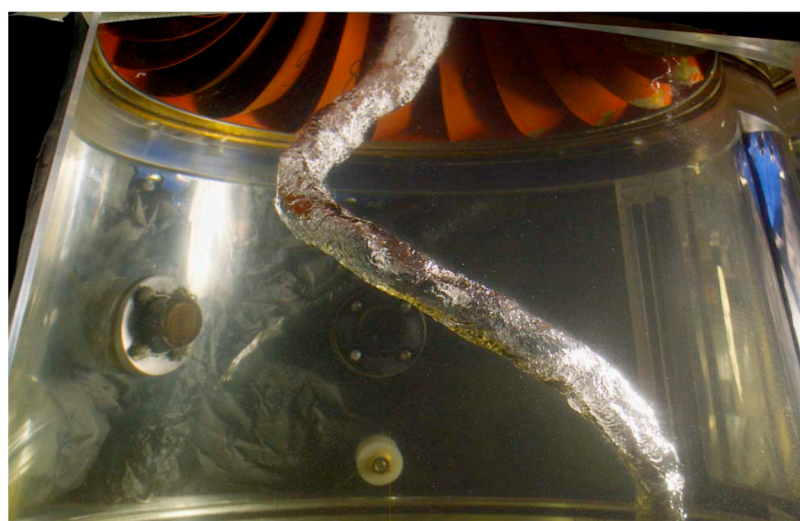
Figure 14. Vapor core rope development for \sigma = 0.380 [41].
