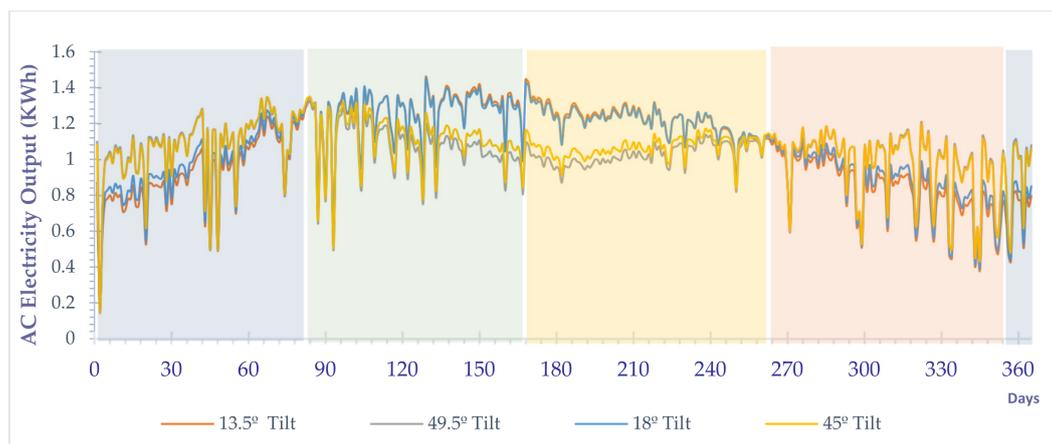
**Figure 7.** Impact of the tilt angle on the PV panel's electricity Output in each season.
