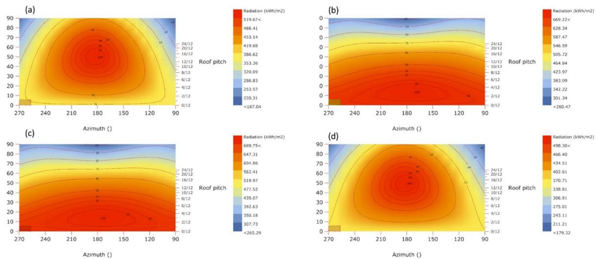
**Figure 6.** The intensity of solar radiation depending on the Photovoltaic panel tilt angle in each season: (a) optimal tilt 49.5 receiving 519 kWh/m<sup>2</sup> during winter; (b) optimal tilt 13.5 receiving 669.22 kWh/m<sup>2</sup> during spring; (c) optimal tilt 13.5 receiving 689 kWh/m<sup>2</sup> during summer; (d) optimal tilt 49.5 receiving 498 kWh/m<sup>2</sup> during the autumn.
