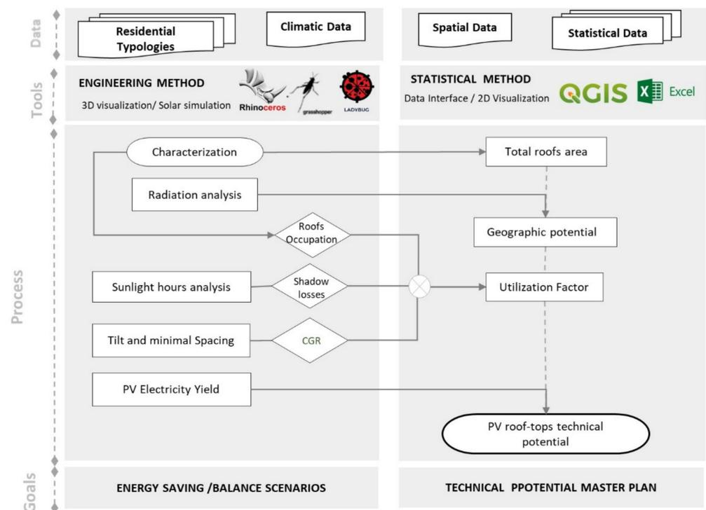
**Figure 1.** Flowchart of the proposed methodology for solar potential assessment.
