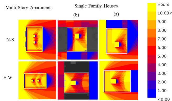
**Figure 5.** Shadows mesh on residential typologies roofs on solstice winter.
