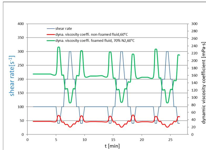
**Figure 4.** Viscosity of non-foamed FF1A and N<sub>2</sub>-foamed FF1B fluid of 70% quality at 60 °C.
