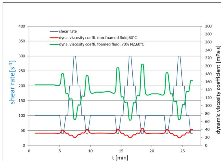
**Figure 5.** Viscosity of non-foamed FF2A and N<sub>2</sub>-foamed FF2B fluid of 70% quality at 60 °C.
