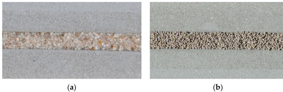
Figure 2. The photo of the fracture filled with quartz sand 20–40 mesh (a), and light ceramic proppant 20–40 mesh (b), with a surface concentration of 9.76 kg/m<sup>2</sup>, between two Ohio sandstone rock blocks, before compressing it on the hydraulic press.
