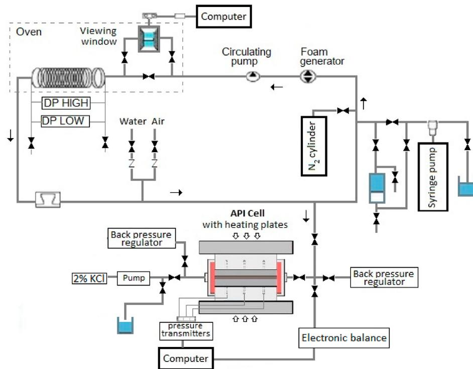
Figure 3. The simplified diagram of the measurement unit for testing the fracture conductivity and damaging it by foamed fracturing fluids.
