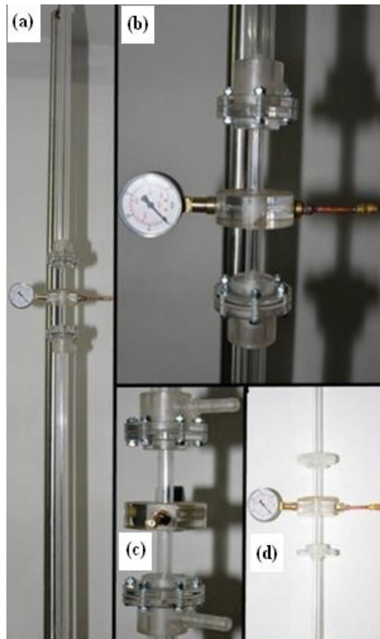
Figure 4. A 1769 mm long heat pipe made of polycarbonate: (a) complete heat pipe, (b,c) isothermal part of the heat pipe, (d) heat pipe without flow exchangers.
