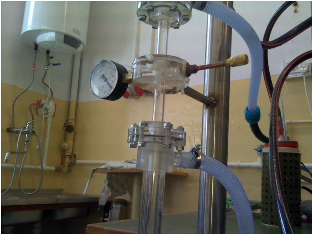
Figure 19. Photo of heat pipe during operation showing evaporation process.
