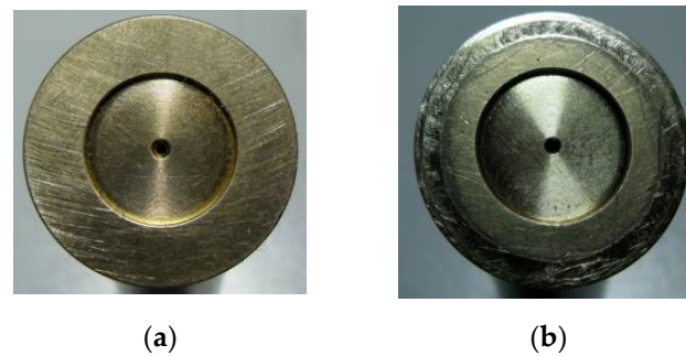
Figure 1. Pictures of slipper eccentric abrasion, where (a) is before eccentric abrasion; (b) is after eccentric abrasion.
