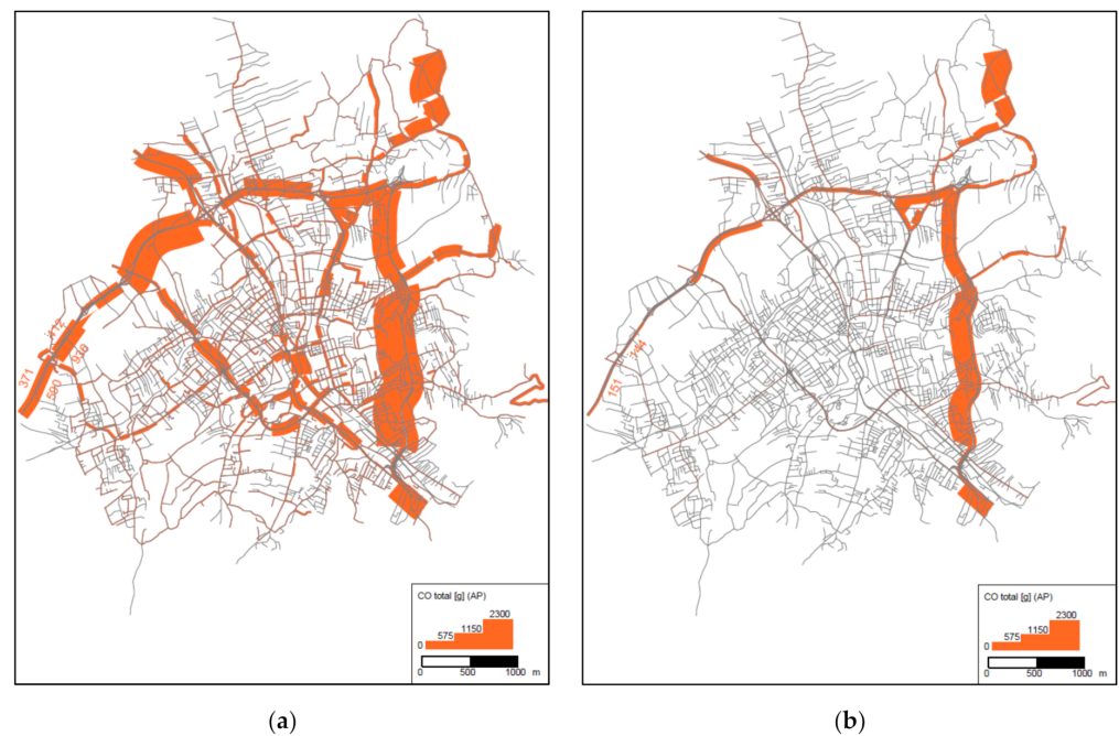
Figure 6. The assessment of CO total [g] (measure from Group 1) for scenario W0 and optimal scenario (W4)—analysis for the whole city: (a) measure for scenario W0; (b) measure for scenario W4.
