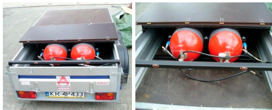
**Figure 10.** View of the transport trailer with cylinders containing treated biogas, with mounting (archives of the Institute of Technology and Life Sciences).
