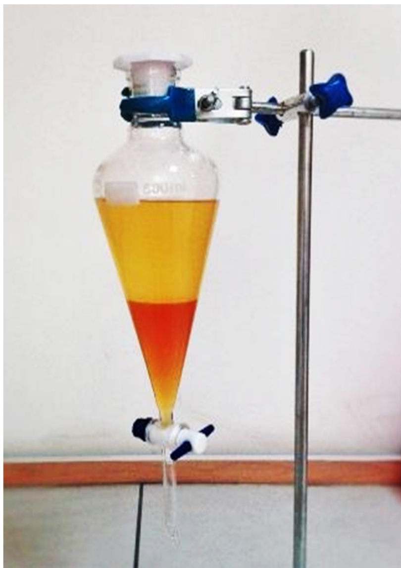
Figure 3. A mixture of methyl ester and glycerin after transesterification reaction.
