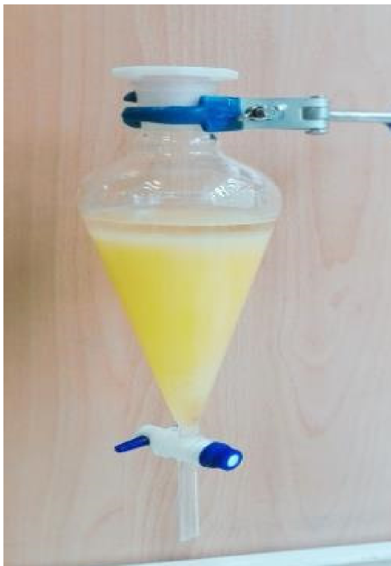
Figure 2. A prepared sample placed in separating funnel after the esterification process.
