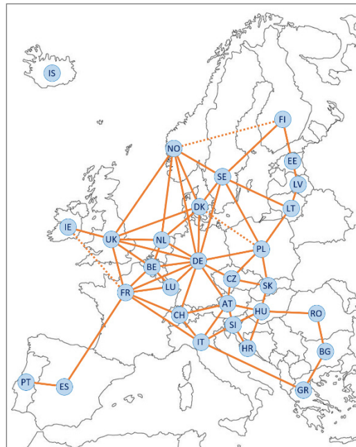
Figure 2. Geographical scope of the unit commitment economic dispatch (UCED) model. Dotted lines represent transmission connections that are not (yet) built in every scenario-year. Cross-border exchanges with the surrounding area (e.g., Russia, Turkey and the non-EU countries in the Balkan region) are neglected, given the fact they are responsible for less than 1% of electricity consumed in the modelled region [55].
