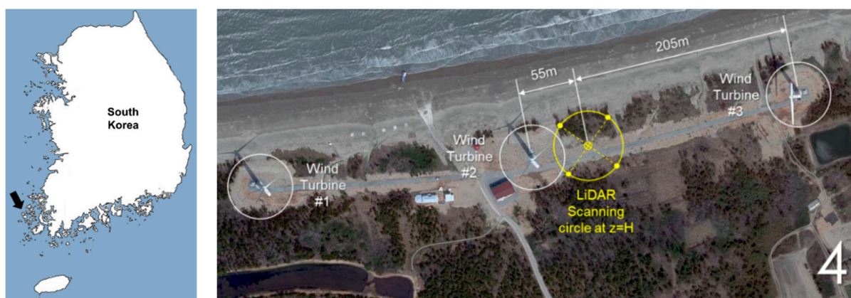
Figure 2. Location (left) and layout (right) of the Shinan wind farm (the wind turbines and the LiDAR).
