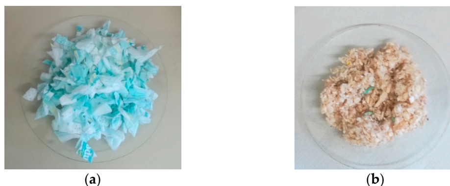
Figure 1. Coarsely shredded diapers (AHPam) (a); cellulosic fraction of sterilized diapers (AHPus) (b).
