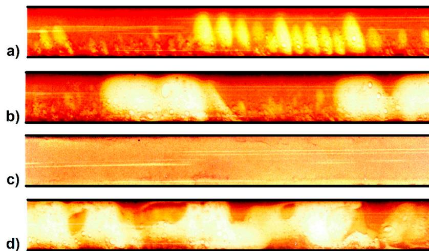
**Figure 2.** Selected two-phase liquid–liquid flow structures in a tube with a diameter of 12 mm (photos from the author’s archive) (a) water droplets in oil, (b) plugs and drops of water in oil, (c) water dispersion in oil, (d) film-dispersed flow of phases.
