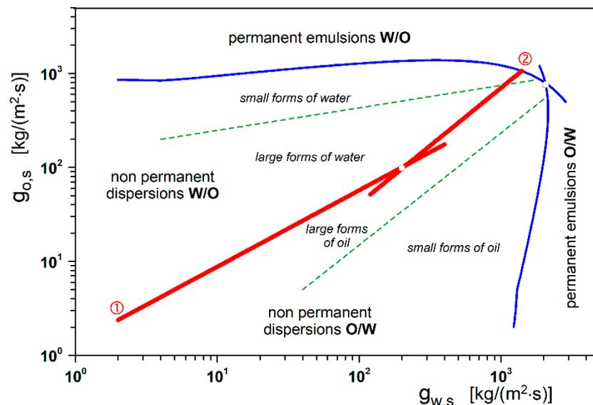
**Figure 1.** Simplified map with two-phase liquid–liquid flow structures with boundaries of phase inversion (red lines) and conditions responsible for generation of non-permanent emulsions (blue lines).
