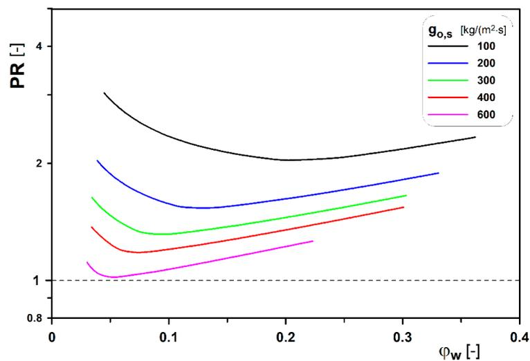
Figure 8. Variations in  $PR$  index for oil with the viscosity of  $\eta_r = 25$ .
