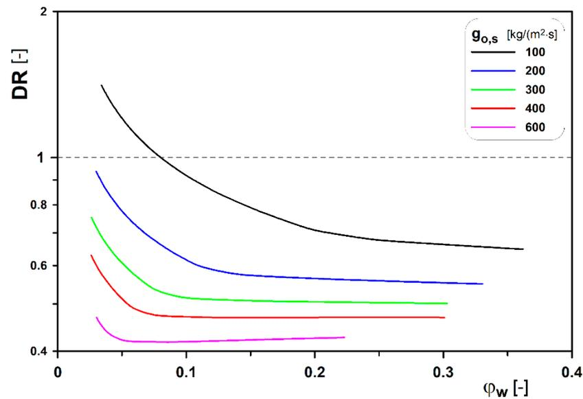
Figure 5. Variations in the  $DR$  index for oil with a viscosity of  $\eta_r = 100$ .
