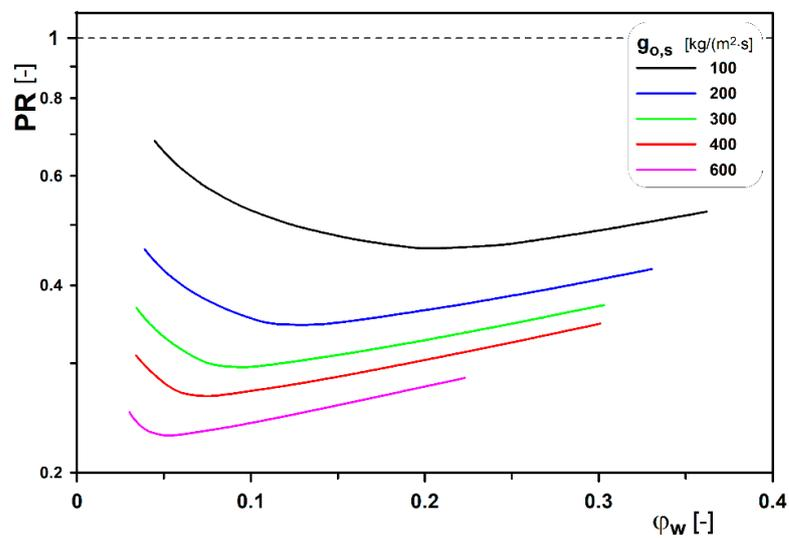
Figure 10. Variations in  $PR$  index for oil with the viscosity  $\eta_r = 300$ .
