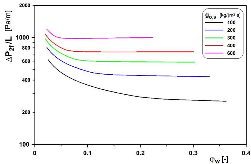
Figure 4. Variations in flow resistance for water–oil mixture recorded for  $\eta_r = 300$ .
