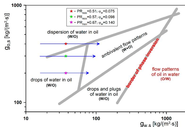
Figure 12. Selected series of simulations for  $\eta_r = 100$  vs. two-phase liquid–liquid flow structures.
