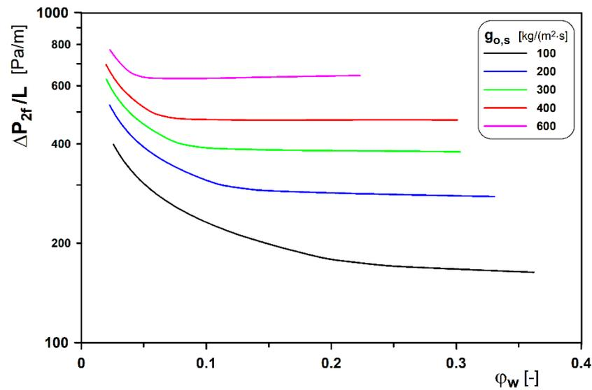
Figure 3. Variations in resistance of oil-water flow recorded for  $\eta_r = 100$ .
