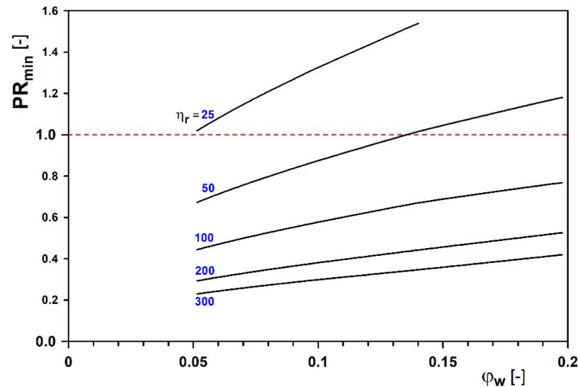
Figure 11. Smallest viable values of PR for oils with various viscosities.
