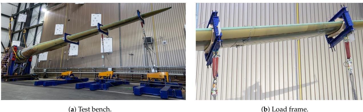
**Figure 1.** Experimental setup for load case Mymax by Fraunhofer IWES [8].
