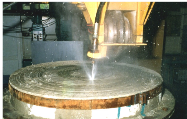
Figure 14. The view of concrete sample cutting using HPW jet: d = 0.8 mm, L = 70 mm, p = 60 MPa [1].
