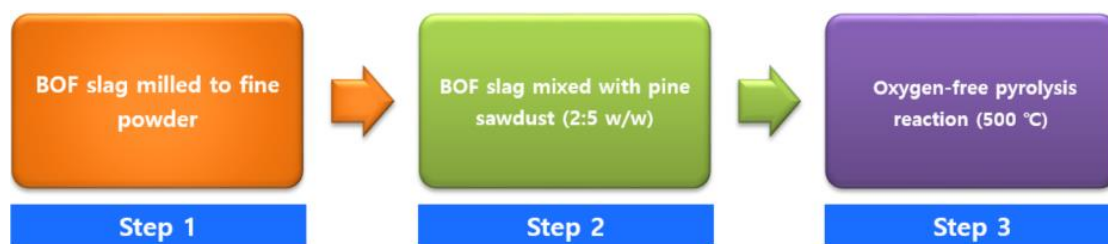
Figure 1. Preparation of MSSB from BOF slag and pine sawdust.
