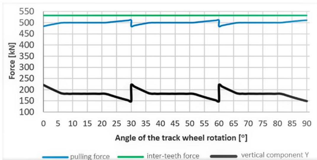
**Figure 20.** Diagram of changes in the following forces: pulling force, inter-teeth force, and vertical component Y in a function of track wheel rotation angle.
