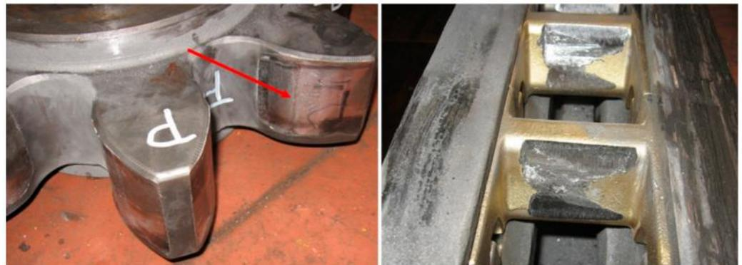
**Figure 4.** Damages to the track wheel and the Flextrack racks during the field tests.
