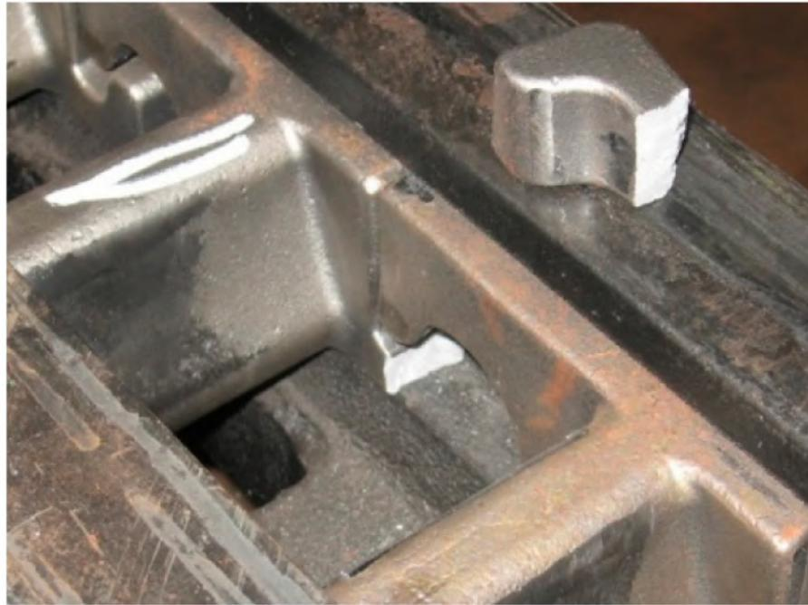
**Figure 21.** View of one of the damaged toothed segments of the Komtrack system.
