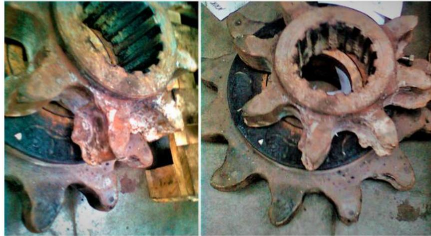
**Figure 2.** Damaged track wheels of the Eicotrack system.
