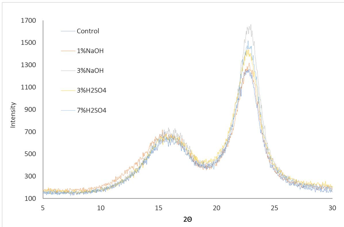
**Figure 6.** X-ray diffraction pattern of corncob cellulose before and after pretreatment.
