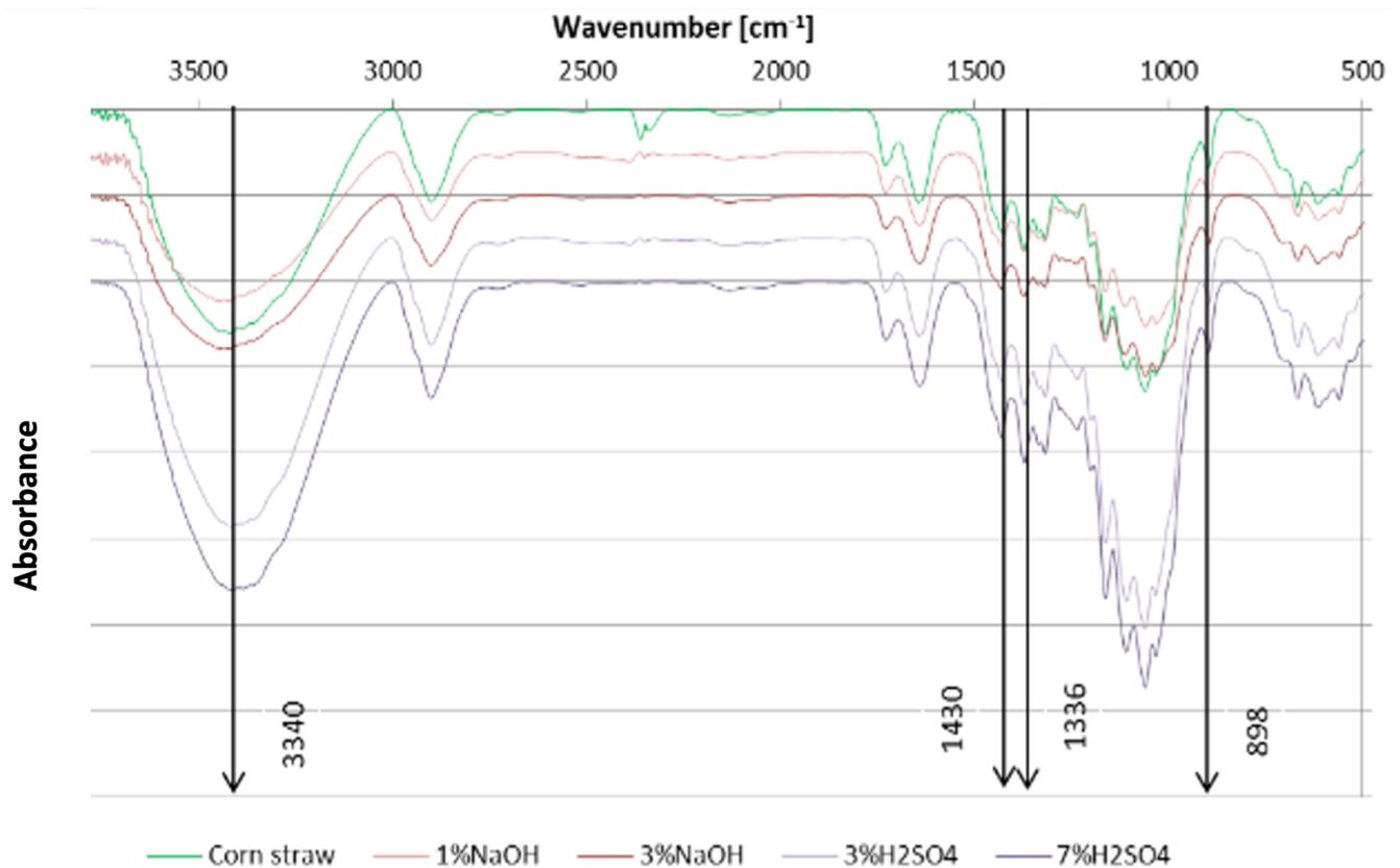
Figure 4. FTIR spectrum of corn straw cellulose before and after pretreatment.
