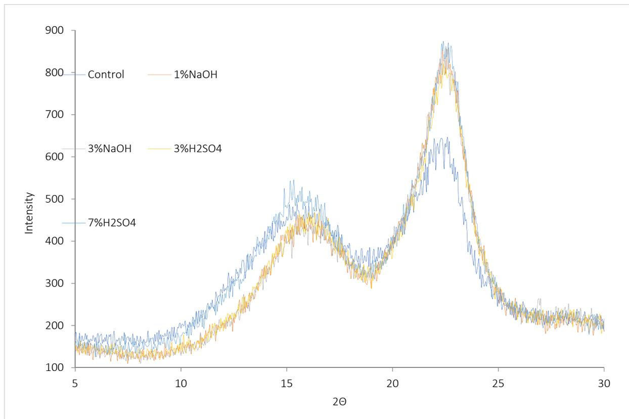
**Figure 7.** X-ray diffraction pattern of corn straw cellulose before and after pretreatment.
