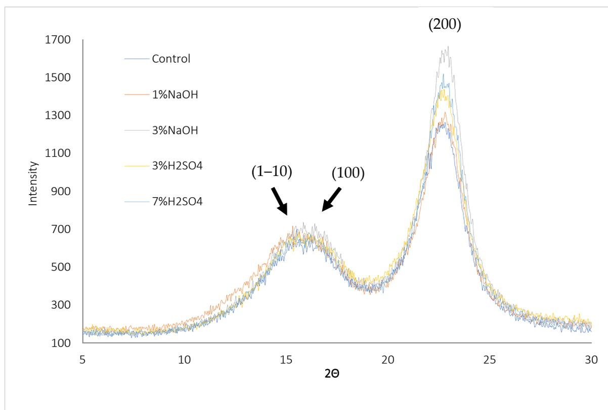
**Figure 5.** X-ray diffraction pattern of poplar cellulose before and after pretreatment.
