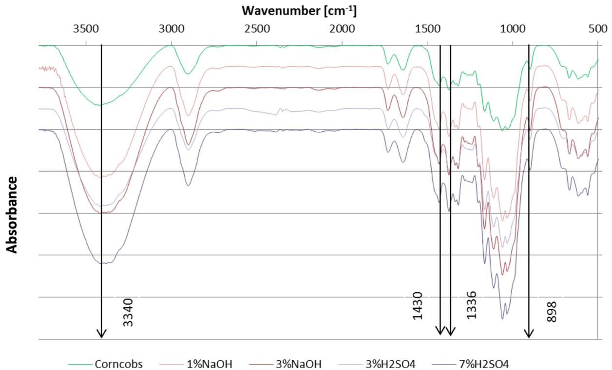
Figure 3. FTIR spectrum of corncob cellulose before and after pretreatment.
