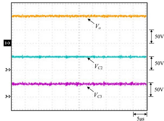
Figure 25. Waveforms measured under the thermoelectric system: (1)  $V_o$ ; (2)  $V_{C2}$ ; (3)  $V_{C3}$ .
