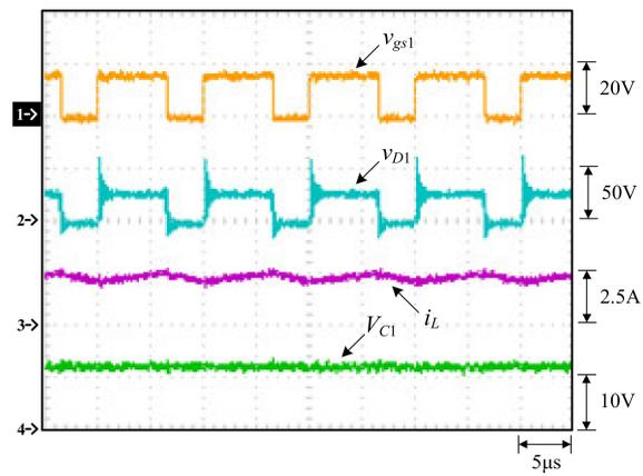
Figure 22. Waveforms measured under the thermoelectric system: (1)  $v_{gs1}$ ; (2)  $v_{D1}$ ; (3)  $i_L$ ; (4)  $V_{C1}$ .
