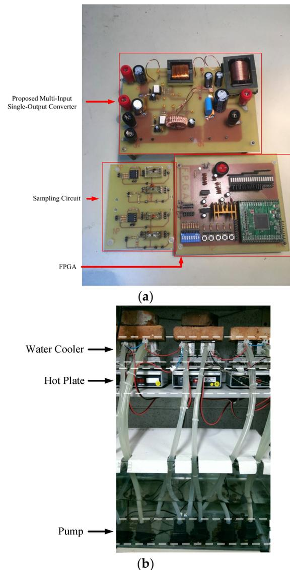
**Figure 27.** Photos of the proposed thermoelectric system: (a) MISOC circuit; (b) thermoelectric platform.
