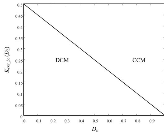
**Figure 14.** Boundary curve between CCM and DCM for  $L_o$ .
