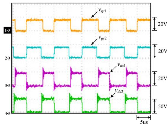
**Figure 21.** Waveforms measured under the thermoelectric system: (1)  $v_{gs1}$ ; (2)  $v_{gs2}$ ; (3)  $v_{ds1}$ ; (4)  $v_{ds2}$ .
