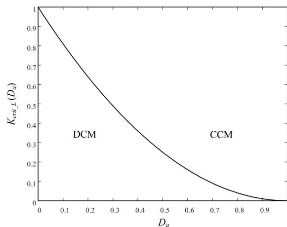
**Figure 11.** Boundary curve between CCM and DCM for  $L$ .
