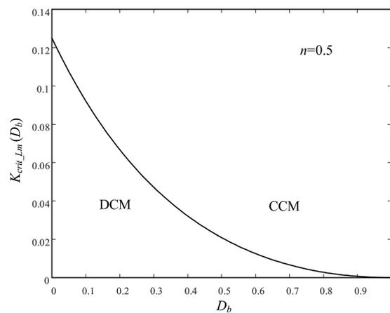
Figure 13. Boundary curve between CCM and DCM for  $L_m$ .
