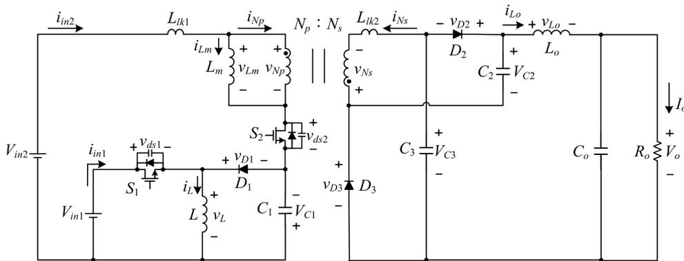
**Figure 5.** Proposed isolated MISOC circuit.
