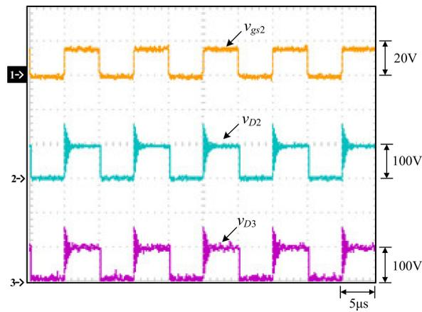
Figure 23. Waveforms measured under the thermoelectric system: (1)  $v_{gs2}$ ; (2)  $v_{D2}$ ; (3)  $v_{D3}$ .
