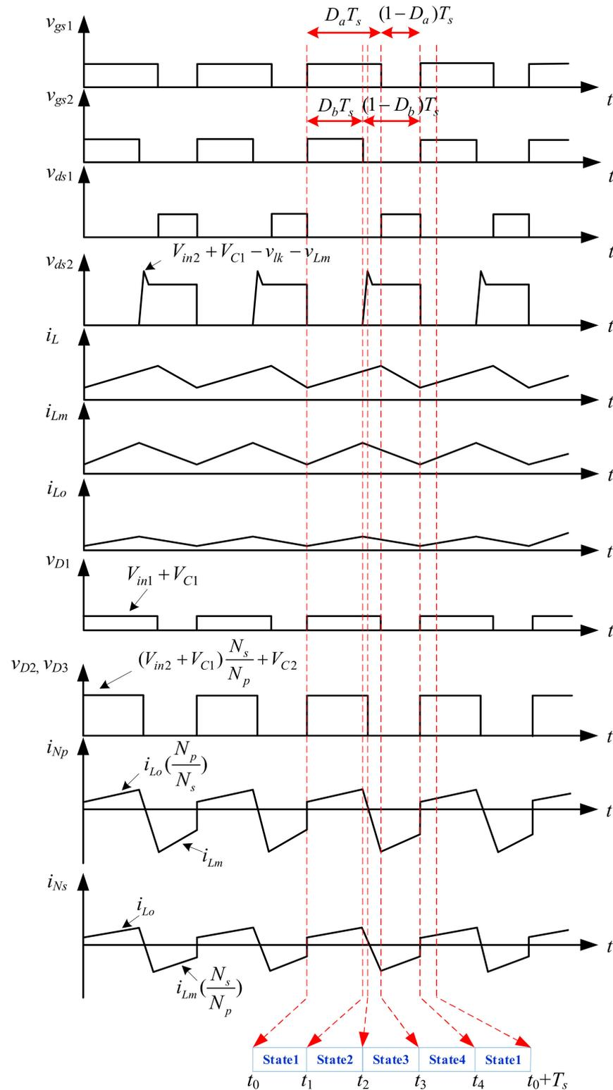
Figure 6. Illustrated waveforms relevant to the proposed isolated MISOC circuit.
