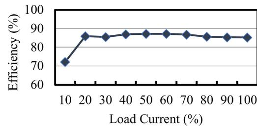
**Figure 20.** Curve of efficiency versus load current.
