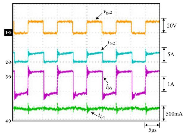
Figure 24. Waveforms measured under the thermoelectric system: (1)  $v_{gs2}$ ; (2)  $i_{in2}$ ; (3)  $i_{Ns}$ ; (4)  $i_{Lo}$ .
