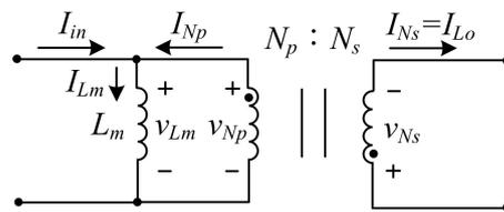
**Figure 12.** Equivalent model for DC current analysis of the coupled inductor.
