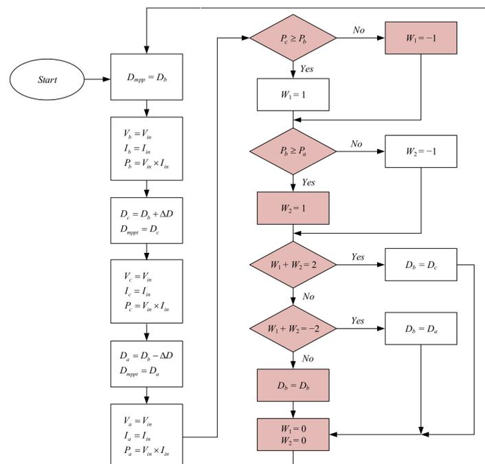
Figure 3. Operating procedure of the three-point weighting strategy for MPPT.
