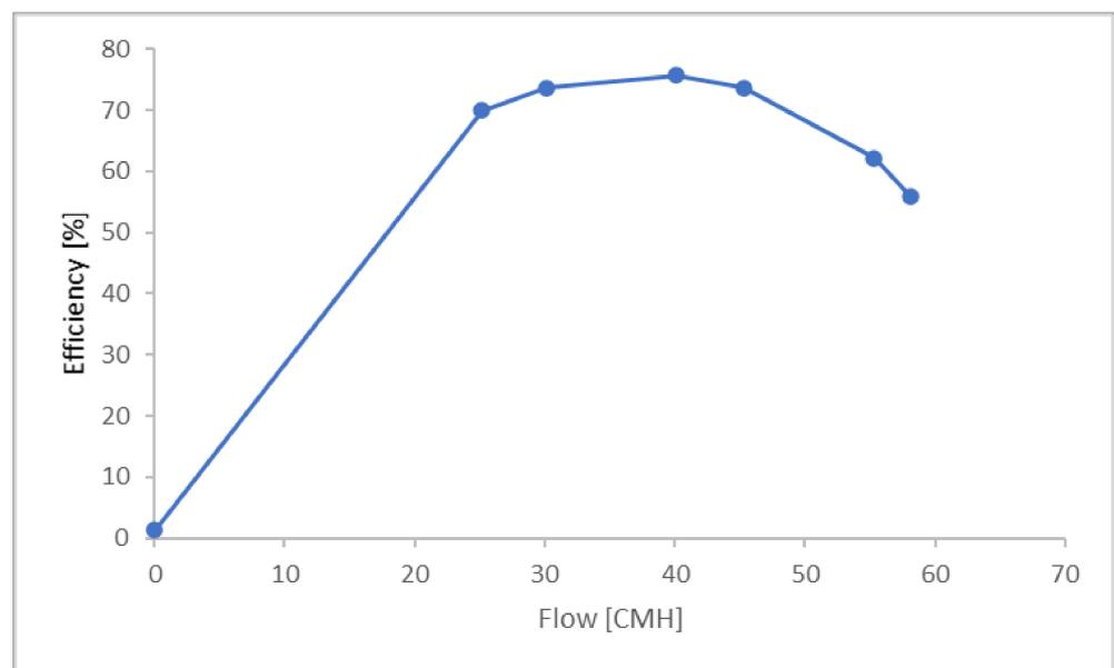
Figure 10. Efficiency pump curve.
