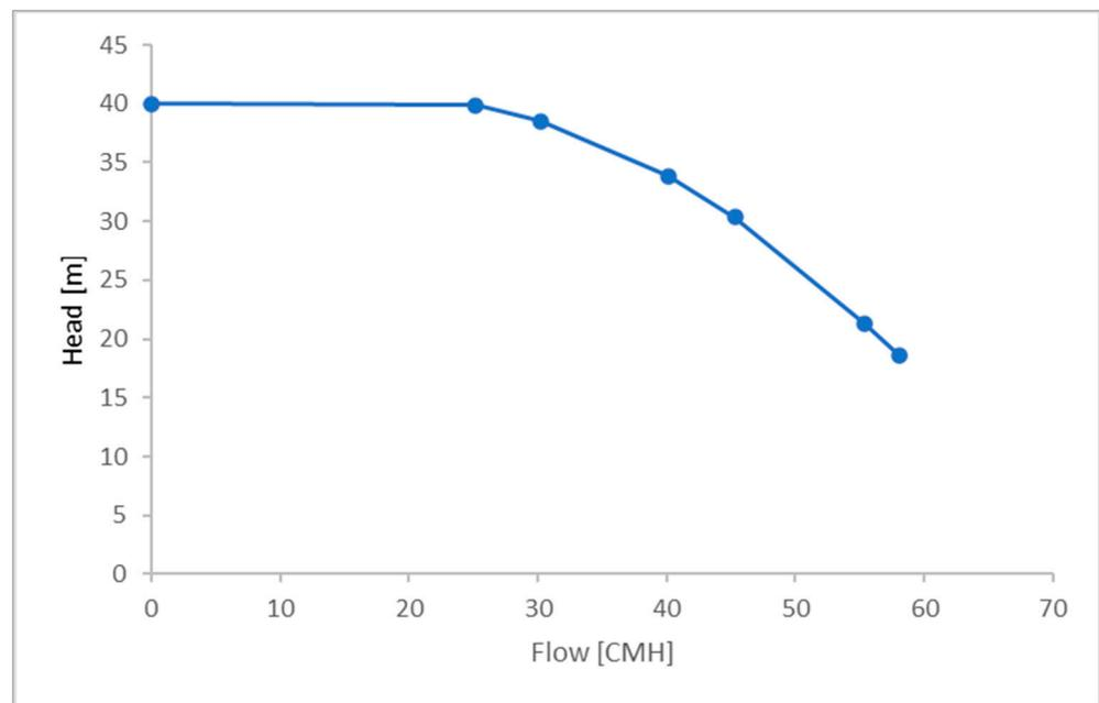
Figure 9. Hydraulic pump curve.
