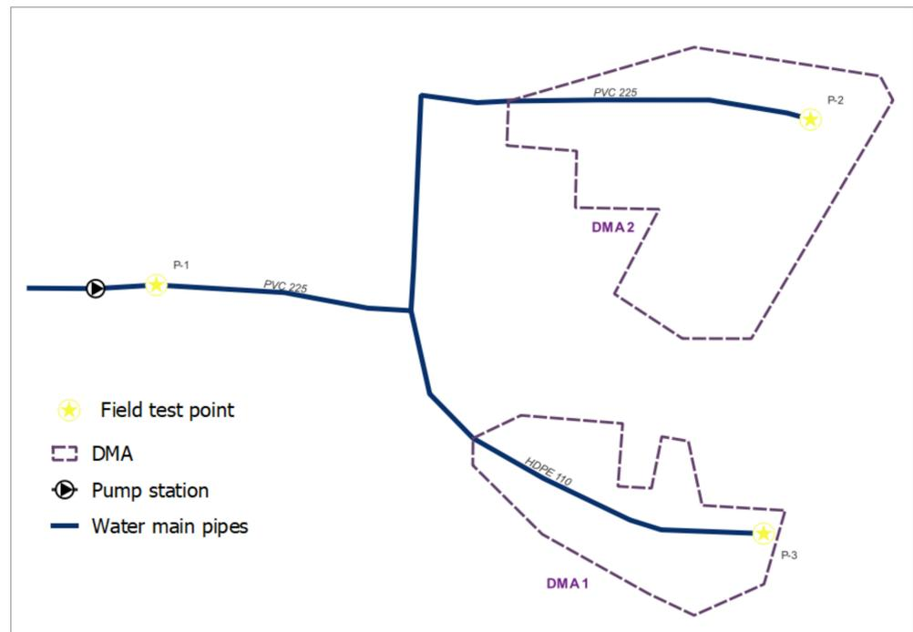
**Figure 3.** Diagram of the analyzed water supply network with division into measurement areas.
