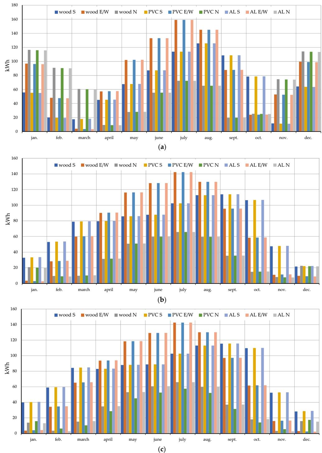
**Figure 10.** Monthly window heat load for Bor as a function of the material and orientation: (a) single-pane fixed window, (b) double-pane window with air filling and (c) double-pane window with argon filling.
