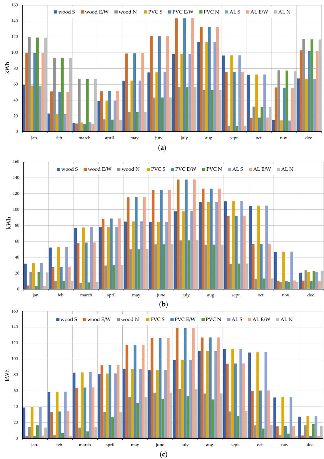
**Figure 11.** Monthly window heat load for Žilina as a function of the material and orientation: (a) single-pane fixed window, (b) double-pane window with air filling and (c) double-pane window with argon filling.
