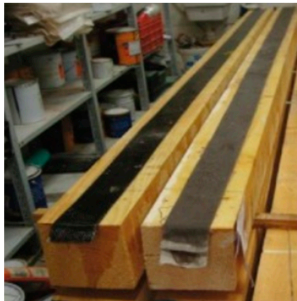
Figure 6. FRP sheet reinforced timber beam [45].
