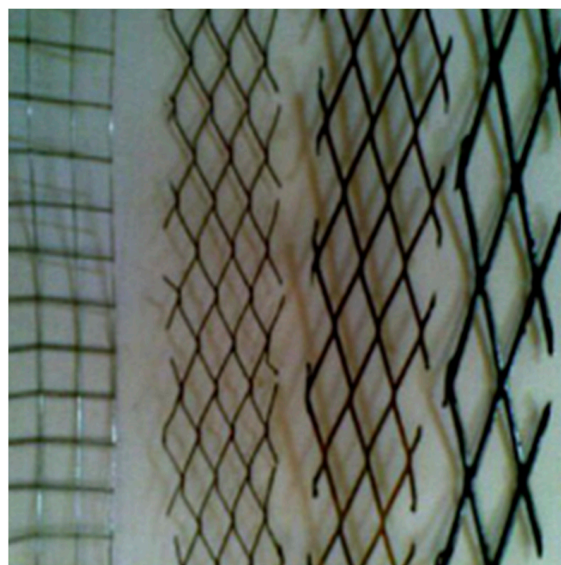
Figure 3. Two shapes of wire mesh for concrete slab experimented by Ibrahim, square shape (left) and diamond shape (right) [27].
