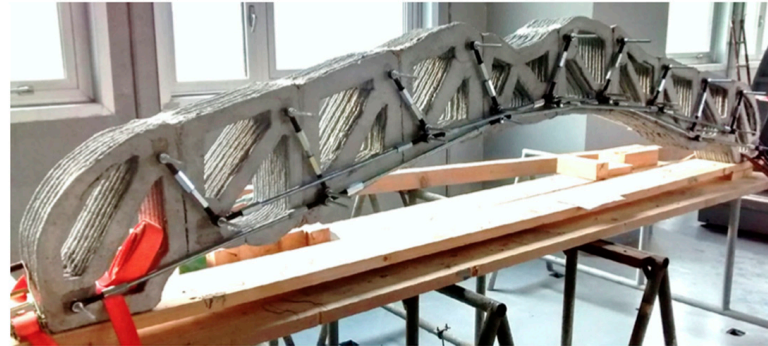
Figure 11. Printed hollow concrete units assembled and reinforced by external steel rebars [52].
