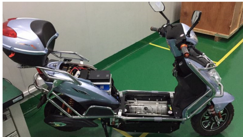
Figure 8. The e-scooter equipped with the passive fuel cell/Li-ion battery hybrid system.
