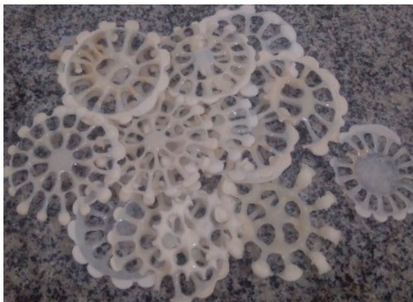
Figure 2. PMMA based dental resins in form of rosettes, discharged by the quality production process control, were used as raw material by depolymerization at 345, 405, and 420 °C, atmospheric pressure, in pilot scale.
