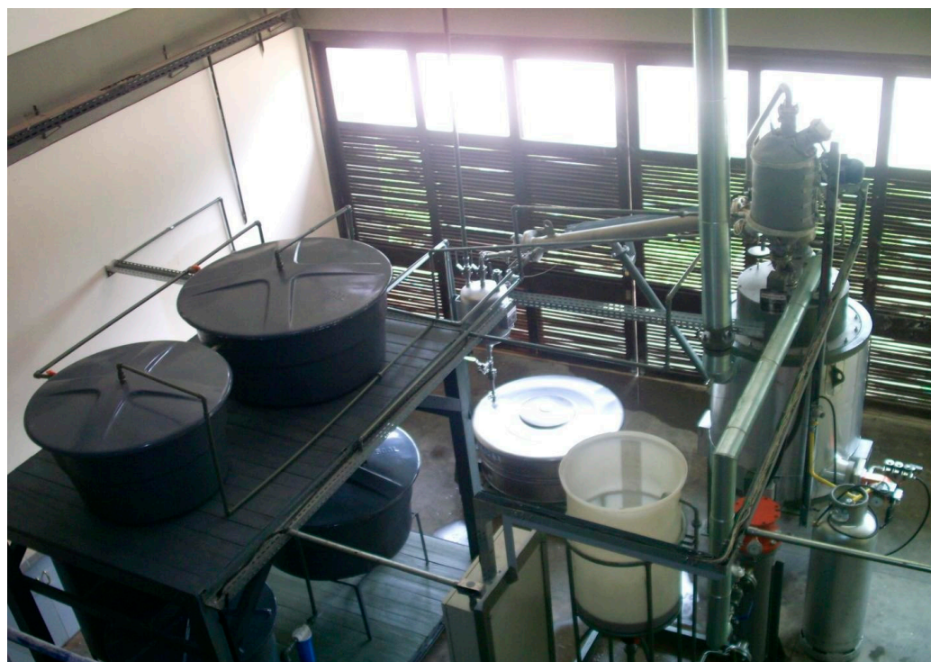
Figure 3. Depolymerization reactor of 143 L for thermic degradation of PMMA resin teeth + fragments of triturated empty rosettes at 345, 405, and 420 °C, atmospheric pressure, in pilot scale.
