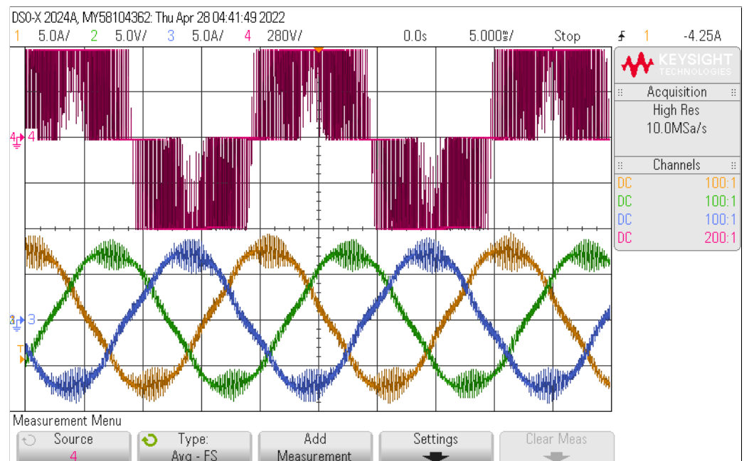
Figure 6. Oscilloscope voltage and current waveforms for the CL HST-SCS.
