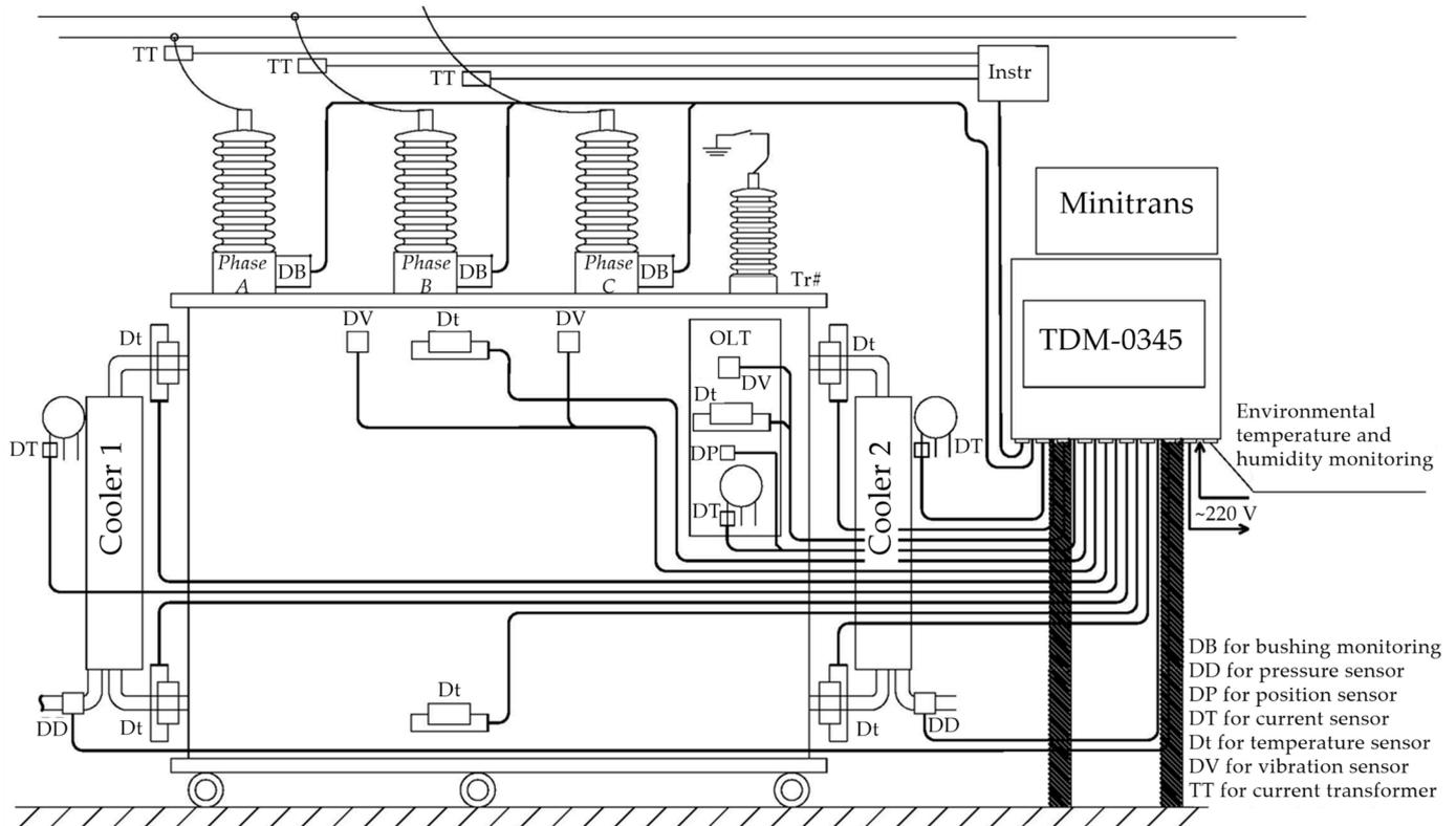
**Figure 2.** Part of the functional diagram of the furnace transformer condition monitoring system.
