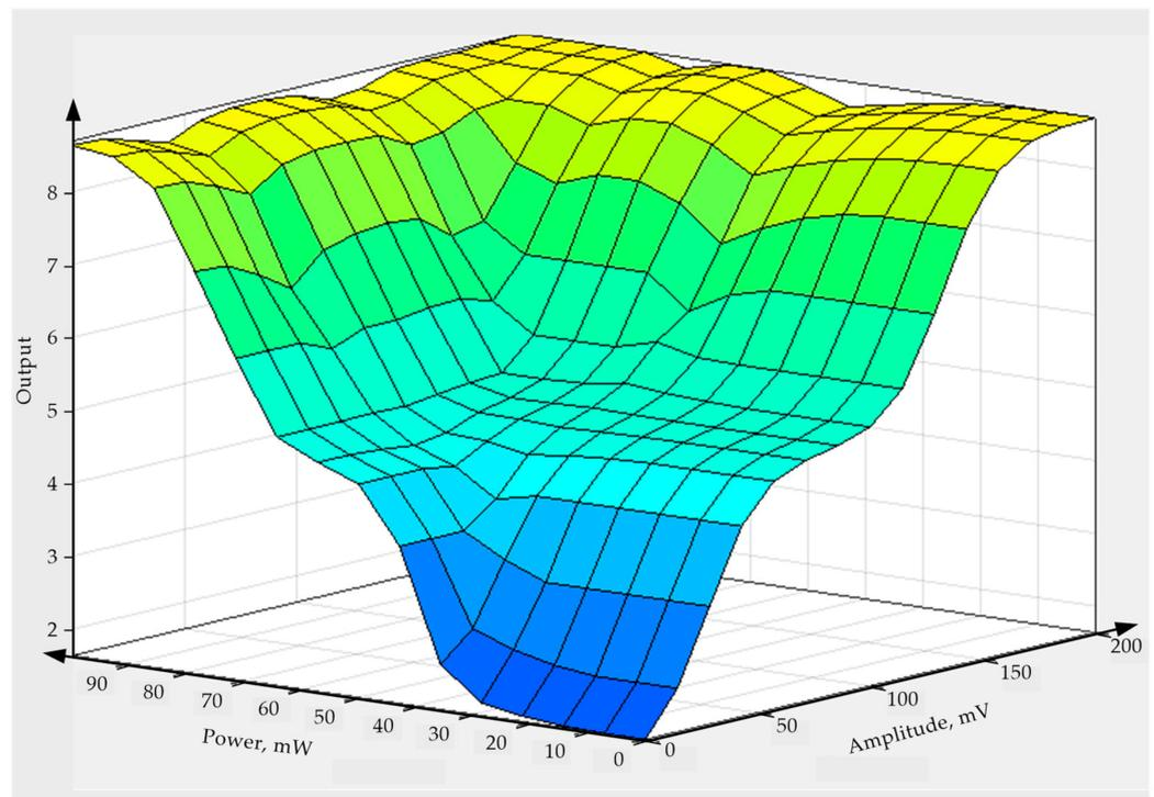
**Figure 6.** This surface shows how *PD* power and amplitude affect the output linguistic variable (in points).
