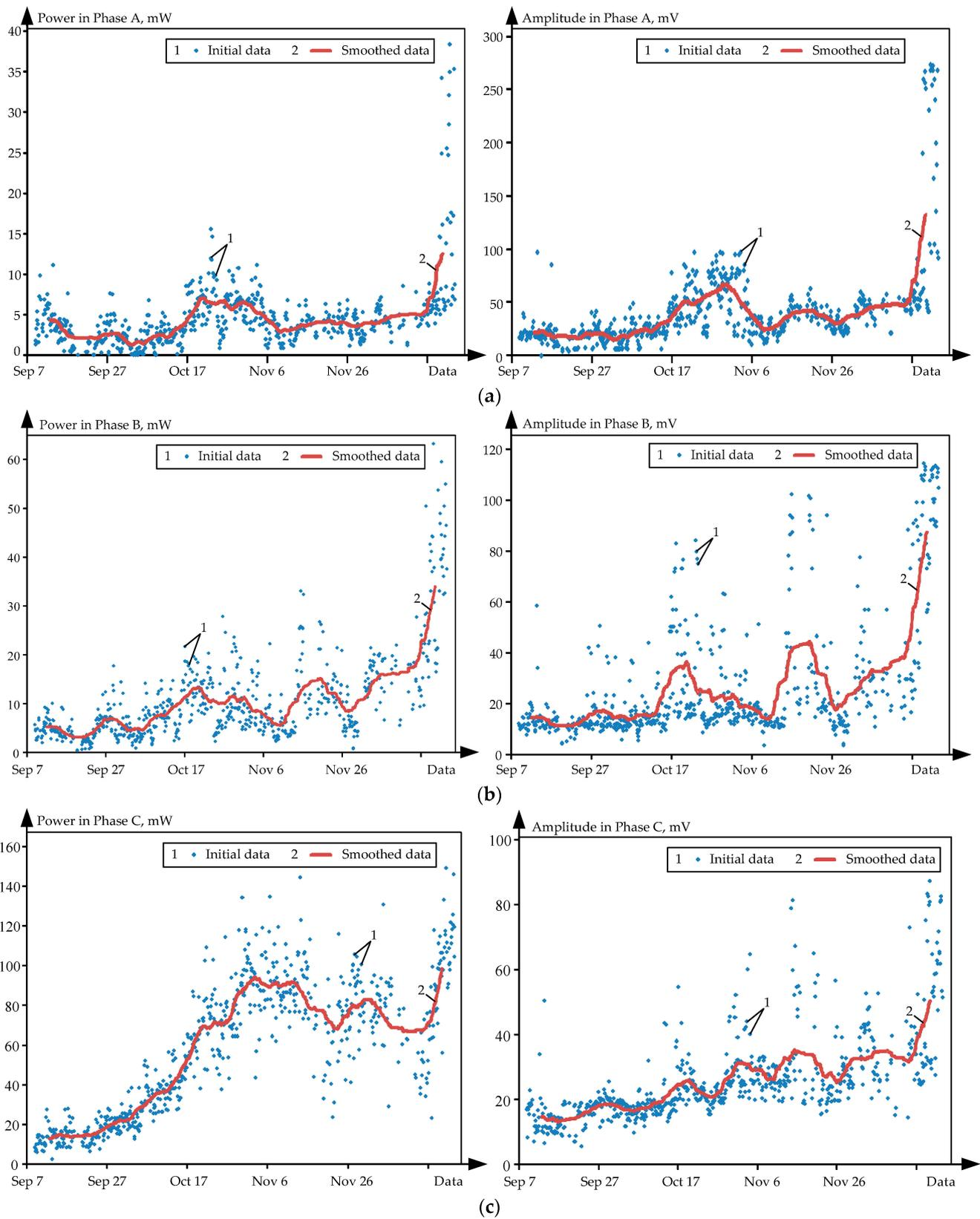
**Figure 7.** Input and smoothed trends of power and amplitude of partial discharges from 9 September to 22 December 2016: (a)—Phase A; (b)—Phase B; (c)—Phase C.
