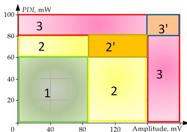
**Figure 4.** Transformer insulation condition assessment based on *PD* readings and using crisp sets: 1 for normal condition; 2 for poor condition; 3 for critical condition; 2' for near-critical condition; 3' for emergency condition.
