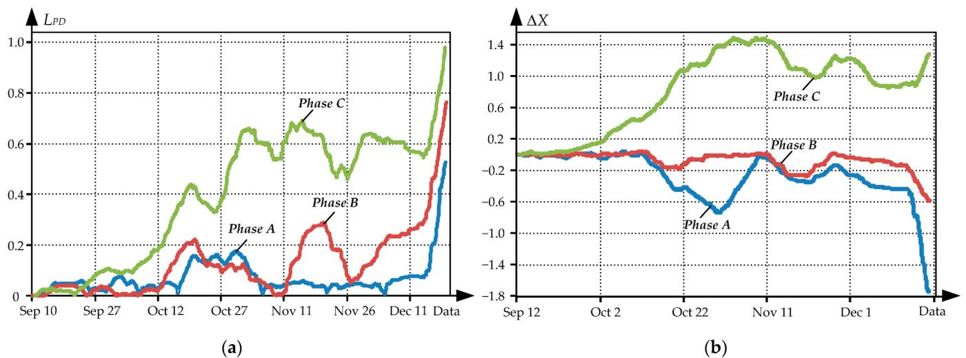
**Figure 9.** Trends in  $L_{PD}$  (a) and  $\Delta X$  (b) from 9 September to 22 December 2016 (defect expansion timeframe).
