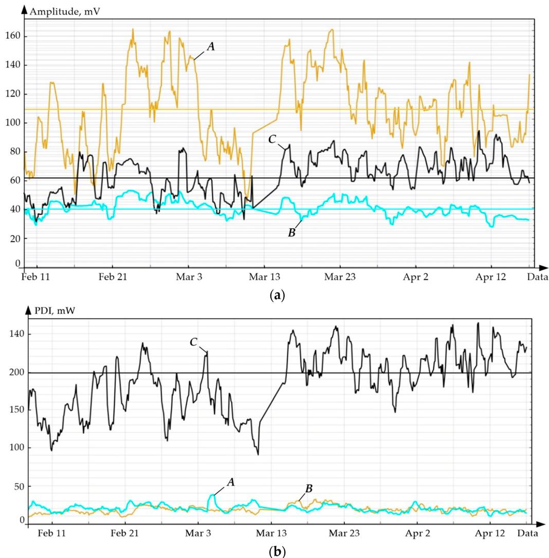
**Figure 3.** Trends in the repeated discharge amplitude (a) and PDI (b) in Phases A, B, C of high-voltage bushings.
