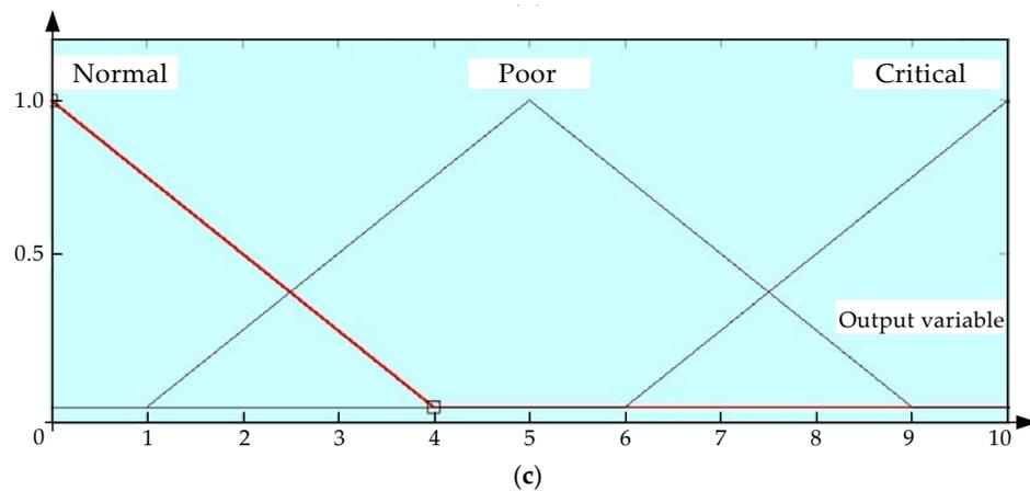
**Figure 5.** Membership functions for the input variables: *Maximum PD Amplitude* (a); *PD Power* (b); and for the output variable *Insulation Condition* (c).
