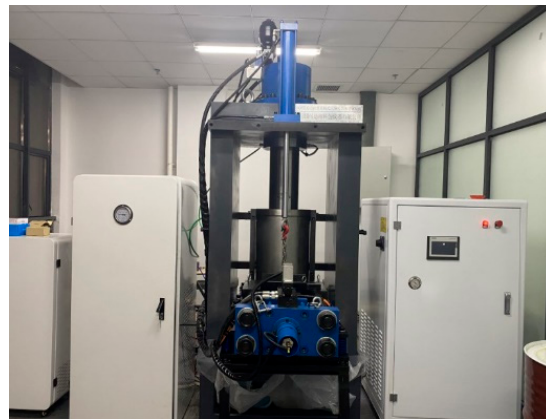
Figure 2. DSZ-1000 mechanical experimental system.
