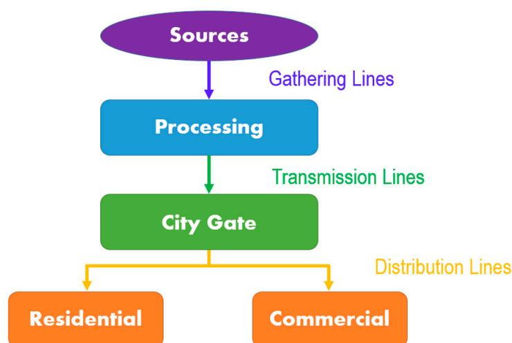
**Figure 4.** Natural gas pipeline network diagram.
