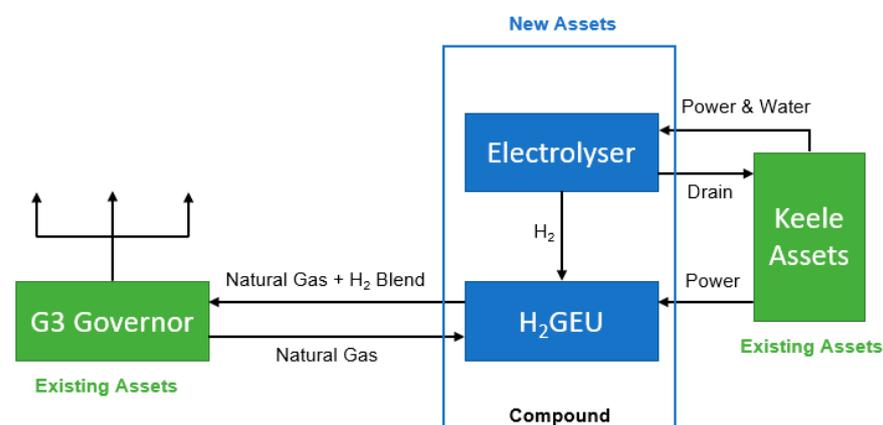
Figure 11. HyDeploy process design flow chart (adapted from [76]).
