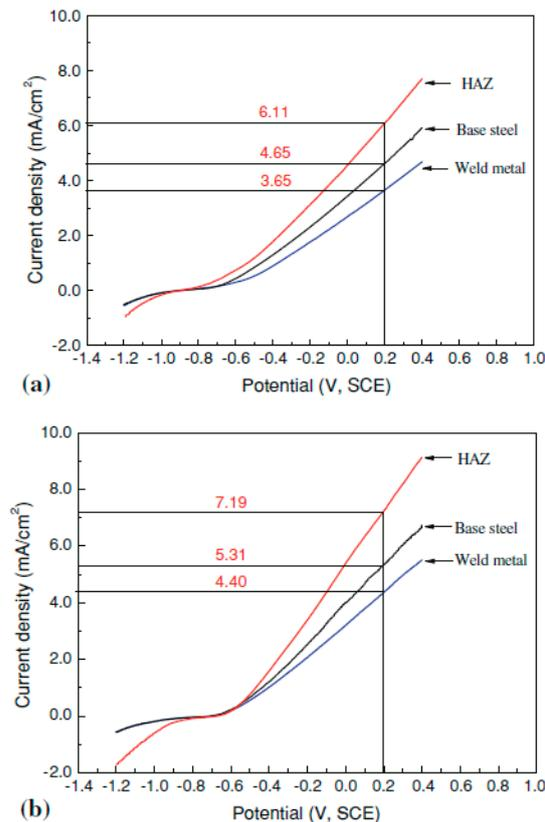
**Figure 10.** Polarization curves measured at various zones of the weld in NS4 solution in the absence (a) and presence (b) of hydrogen-charging at cathodic current density of 10 mA/cm<sup>2</sup> for 2 h [73].
