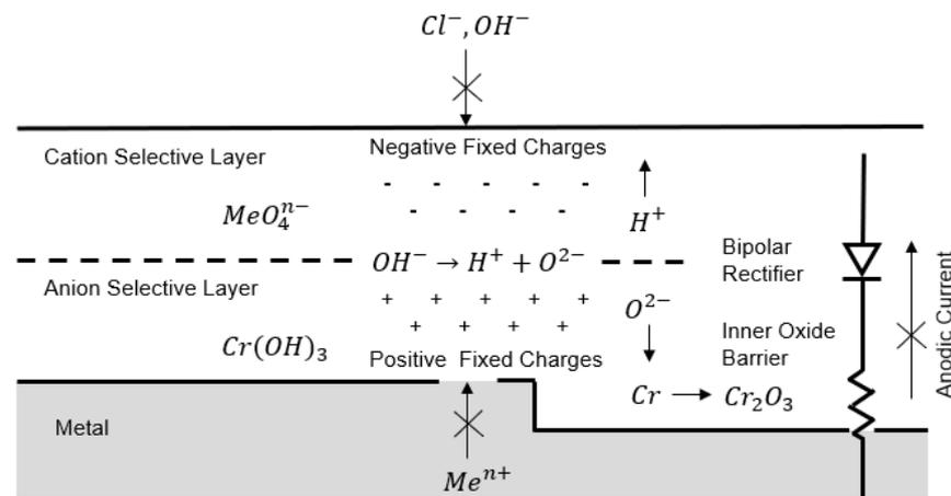
**Figure 8.** Schematic: bipolar passive film model (adapted from [72]).
