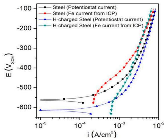
Figure 7. Influence of hydrogen charging on 1018 steel [61].
