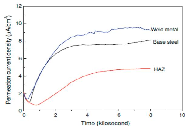
**Figure 9.** Hydrogen permeation current curves [73].
