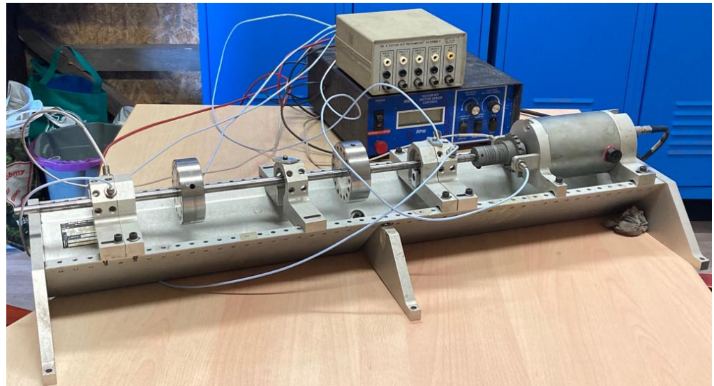
Figure 6. Picture of the Rotor Kit test rig used for model validation.
