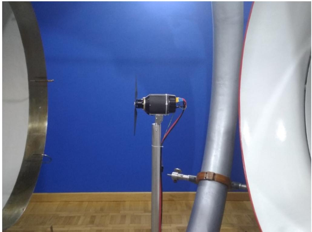
**Figure 6.** Drive unit set at an angle of 90° in relation to the direction of inflow.
