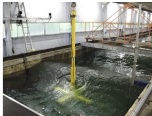
Figure 1. TLP floating offshore wind turbine: the specimen under extreme irregular waves (reprinted from Oguz et al., [5] copyright (2022), LN 5311720742150, with permission from Elsevier).
