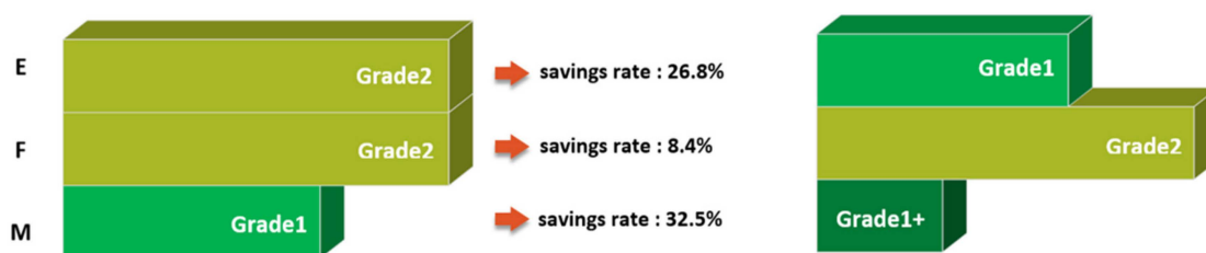
Figure 13. The reduction rate of primary energy consumption per unit area per year and changes in building energy efficiency ratings, due to improvements in windows and ventilation systems.
