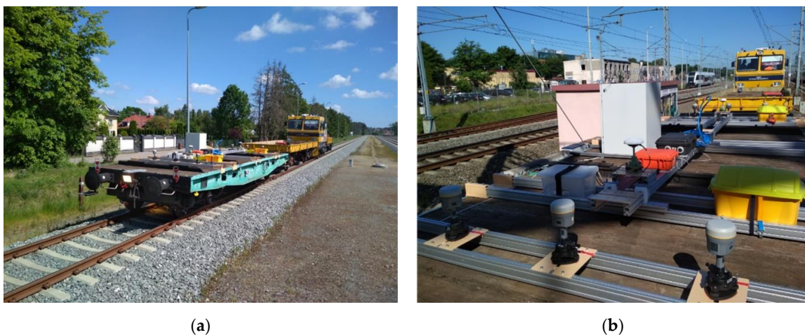
Figure 6. MMP (a) with the equipment used (b) during the railway measurement campaign conducted on 9 June 2021.
