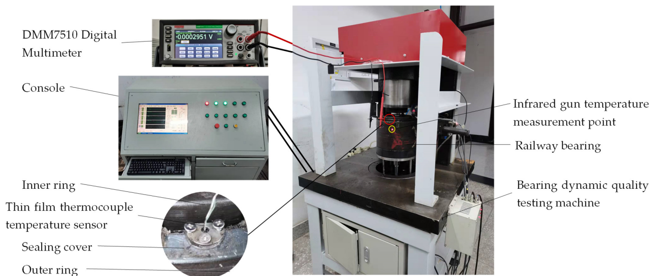
Figure 10. Railway bearing thermal analysis test bench.
