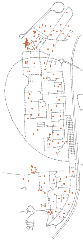
Figure 3. Representation of the graph based on the OpenStreetMaps import to uesgraphs , showing orange dots as detected buildings and grey dots and lines as street nodes and edges.
