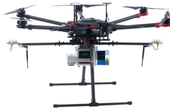
Figure 1. The LiAir 220 drone used for high-resolution image capture of an oil palm tree plantation.
