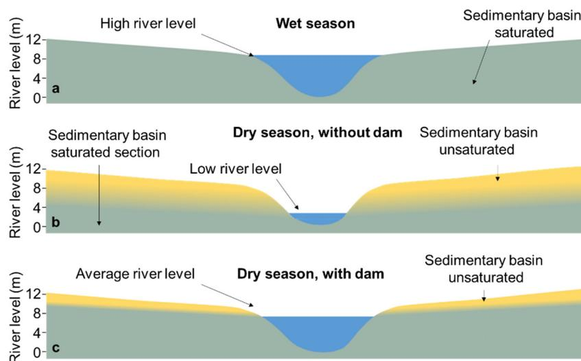
**Figure 8.** Diagram representing the saturation of sedimentary basins and their impact on river level during (a) wet season and (b) dry season without dam, and (c) dry season with the dam.
