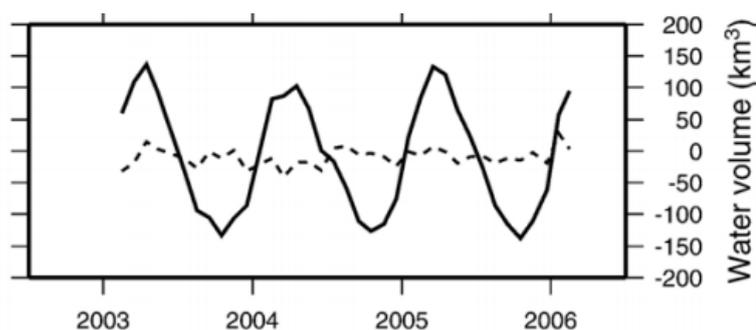
**Figure 3.** Water storage variation in the Tocantins basin (865,000 km<sup>2</sup> area). The solid line is the change in water volume stored in the basin compared to the average. The dotted line is the 12-month average change in water volume stored [26].
