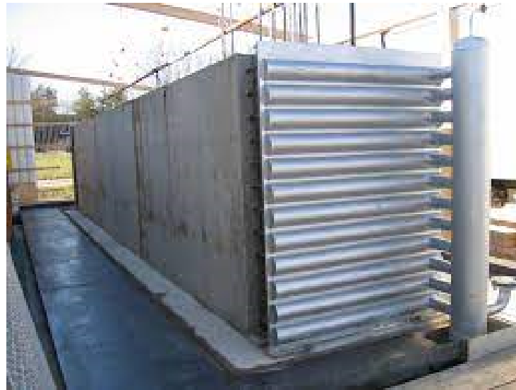
Figure 1. DLR concrete storage concept. Reprinted/adapted with permission from Ref. [9]. 2009, American Society of Mechanical Engineers.
