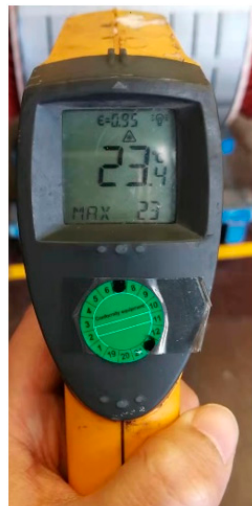
Figure 30. Infrared thermometer to measure shell and shaft.
