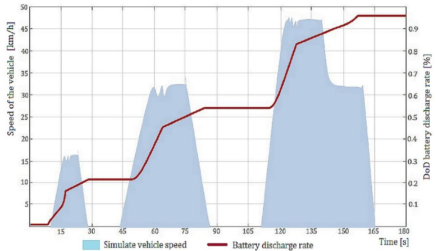
**Figure 15.** Plot of the battery discharge rate and speed of an electric car for a multi-valued logic tree with the floor layout of decision variables of:  $X_5, X_2, X_1, X_4, X_3$ .
