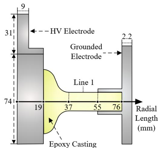
Figure 2. Insulator profile and electrode size.
