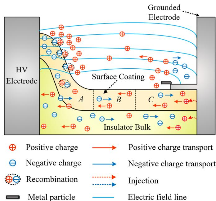
**Figure 11.** Schematic diagram of surface charge accumulation with metal particle adhered to the grounded electrode under negative voltage.
