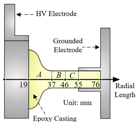
**Figure 4.** Diagram of zoning coating on the insulator surface.
