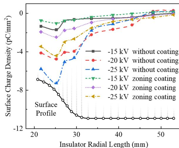
**Figure 7.** Radial distribution of average charge density on insulator surface with and without zoning coating.
