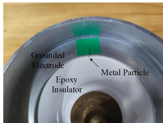
**Figure 8.** Schematic diagram of metal particle placement.
