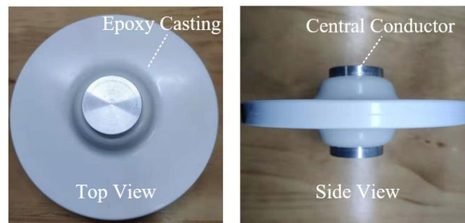
Figure 1. Test insulator.
