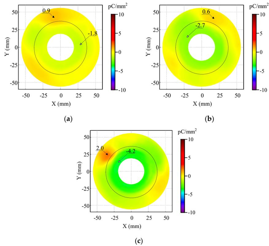
**Figure 6.** Typical charge distribution on insulator with zoning coating under different voltages. (a) Typical charge distribution under  $-15$  kV; (b) Typical charge distribution under  $-20$  kV; (c) Typical charge distribution under  $-25$  kV.
