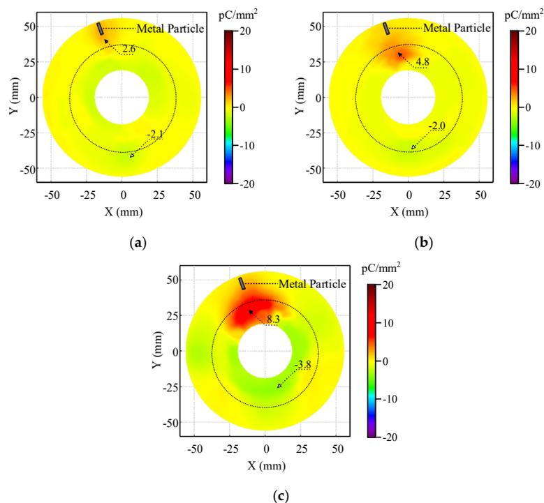
**Figure 10.** Typical charge distribution on the insulator with zoning coating with the metal particle under different voltages. (a) Typical charge distribution under  $-15$  kV; (b) Typical charge distribution under  $-20$  kV; (c) Typical charge distribution under  $-25$  kV.
