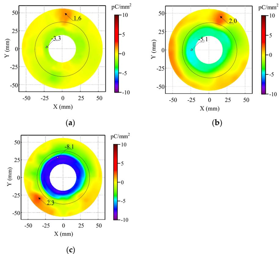
**Figure 3.** Typical charge distribution on insulator without coating under different voltages. (a) Typical charge distribution under  $-15$  kV; (b) Typical charge distribution under  $-20$  kV; (c) Typical charge distribution under  $-25$  kV.
