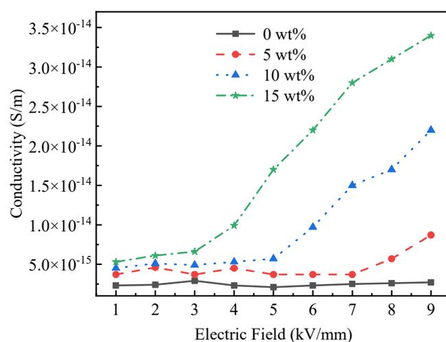
**Figure 5.** Relationship between bulk conductivity and applied electric field of epoxy/SiC coating.
