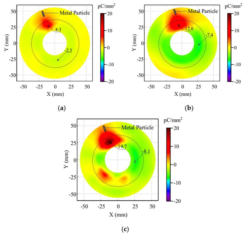
**Figure 9.** Typical charge distribution on the insulator without zoning coating with the metal particle under different voltages. (a) Typical charge distribution under  $-15$  kV; (b) Typical charge distribution under  $-20$  kV; (c) Typical charge distribution under  $-25$  kV.
