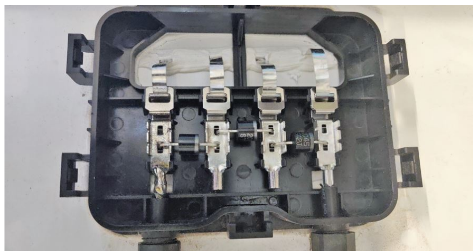
Figure 4. The opened junction box of a BYD 310P6C-36 72 cell PV module, showing the connections of three bypass diodes.
