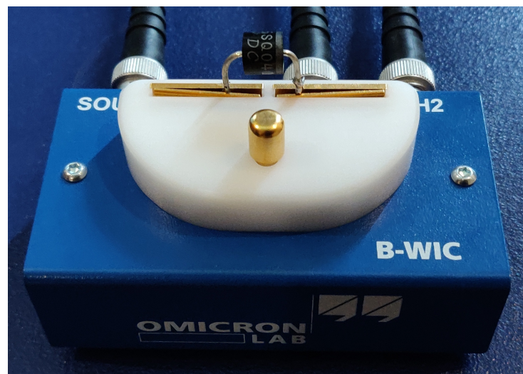
Figure 16. The OMICRON Lab B-WIC impedance adapter for THT components.
