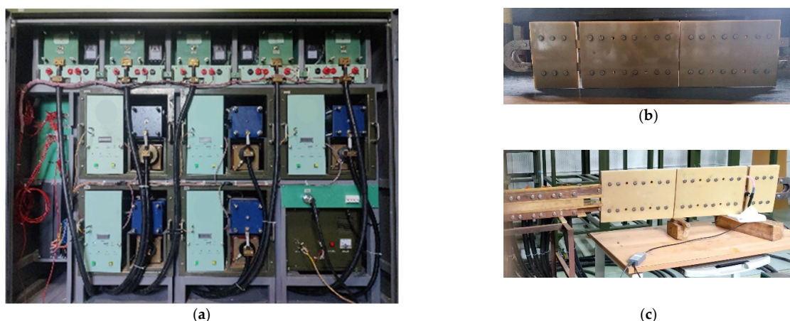
Figure 4. The experiment devices. (a) The capacitive power supply and the charger. (b) The load in experiments. (c) The connection of experimental devices.
