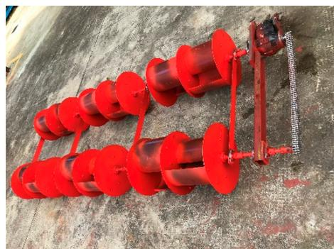
**Figure 2.** Physical model of s-type runner.
