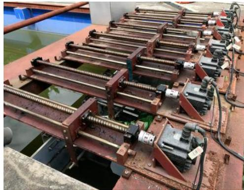
Figure 7. Wave-making system.
