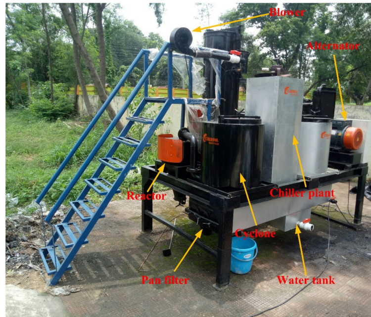
Figure 9. Rear view of the biomass generator [44].
