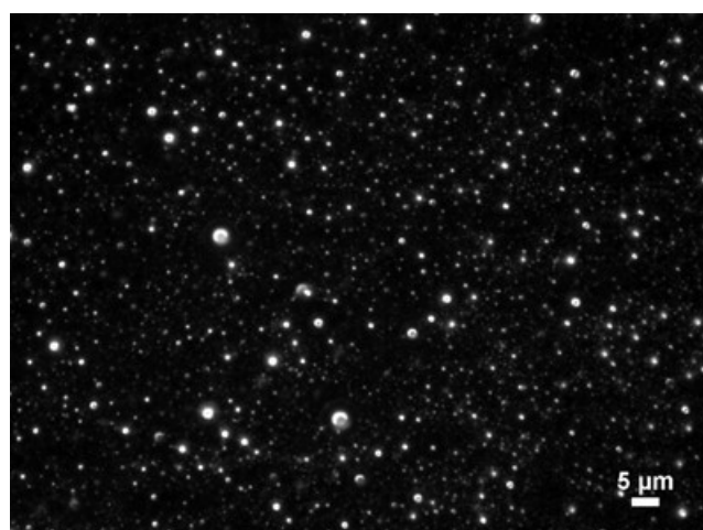
Figure 3. Microscope images for water-in-oil emulsions at 1500 ppm CTAB.
