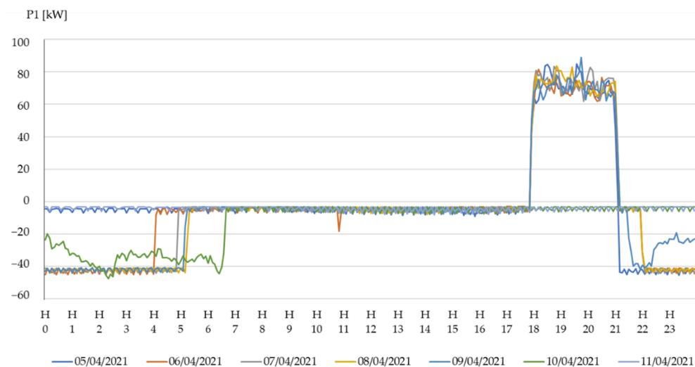
**Figure 5.** BESS active power flow ( $P_1$ ) measured with meter #1 during the week of 5 April 2021 (kW).
