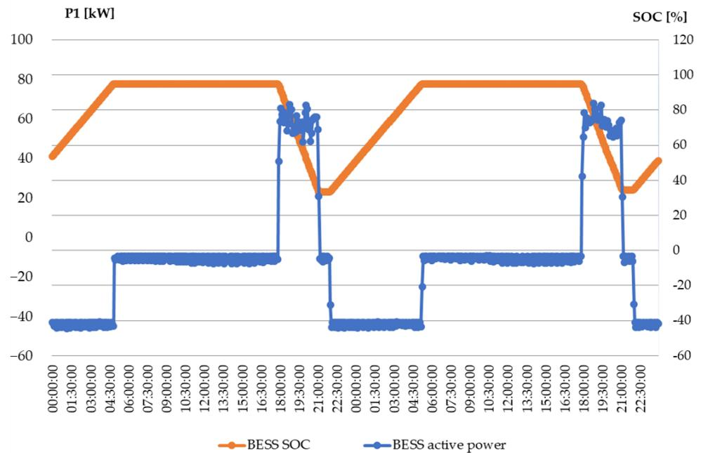
**Figure 6.** BESS active power (P1) and SOC dynamics on 7 April and 8 April 2021.
