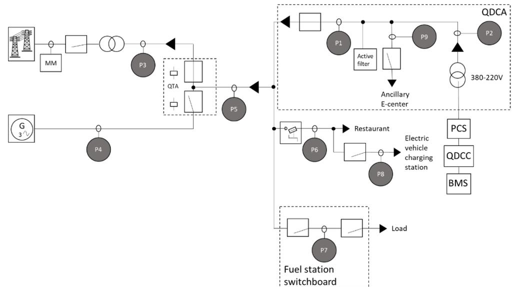
Figure 2. PU single-line diagram adapted from the Supervisory Control and Data Acquisition System (SCADA) [22].
